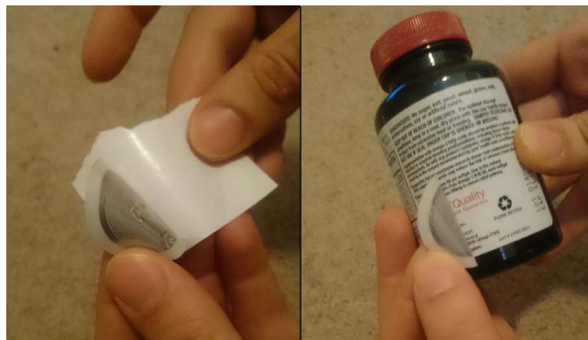
Figure 7. Near Field Communication sample sticky tag with a drug container
