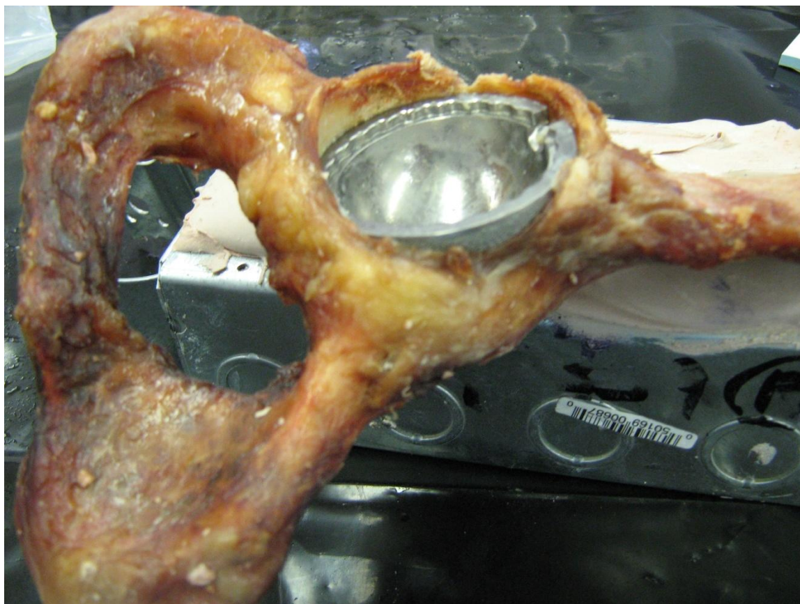
Figure XX. Third control specimen tested. Depuy PINNACLE acetabular cups were press-fit implanted.
