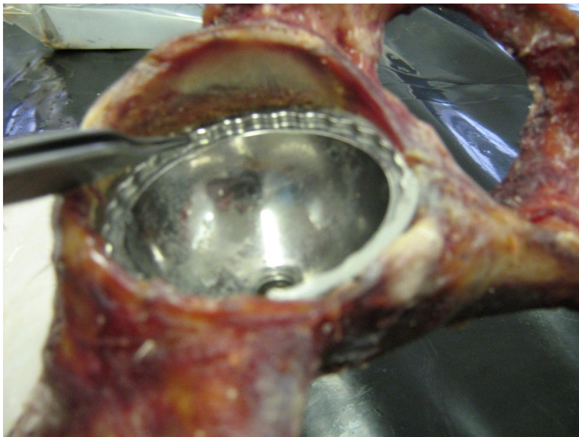
Figure XXI. Second control specimen tested. Depuy PINNACLE acetabular cups were press-fit implanted.
