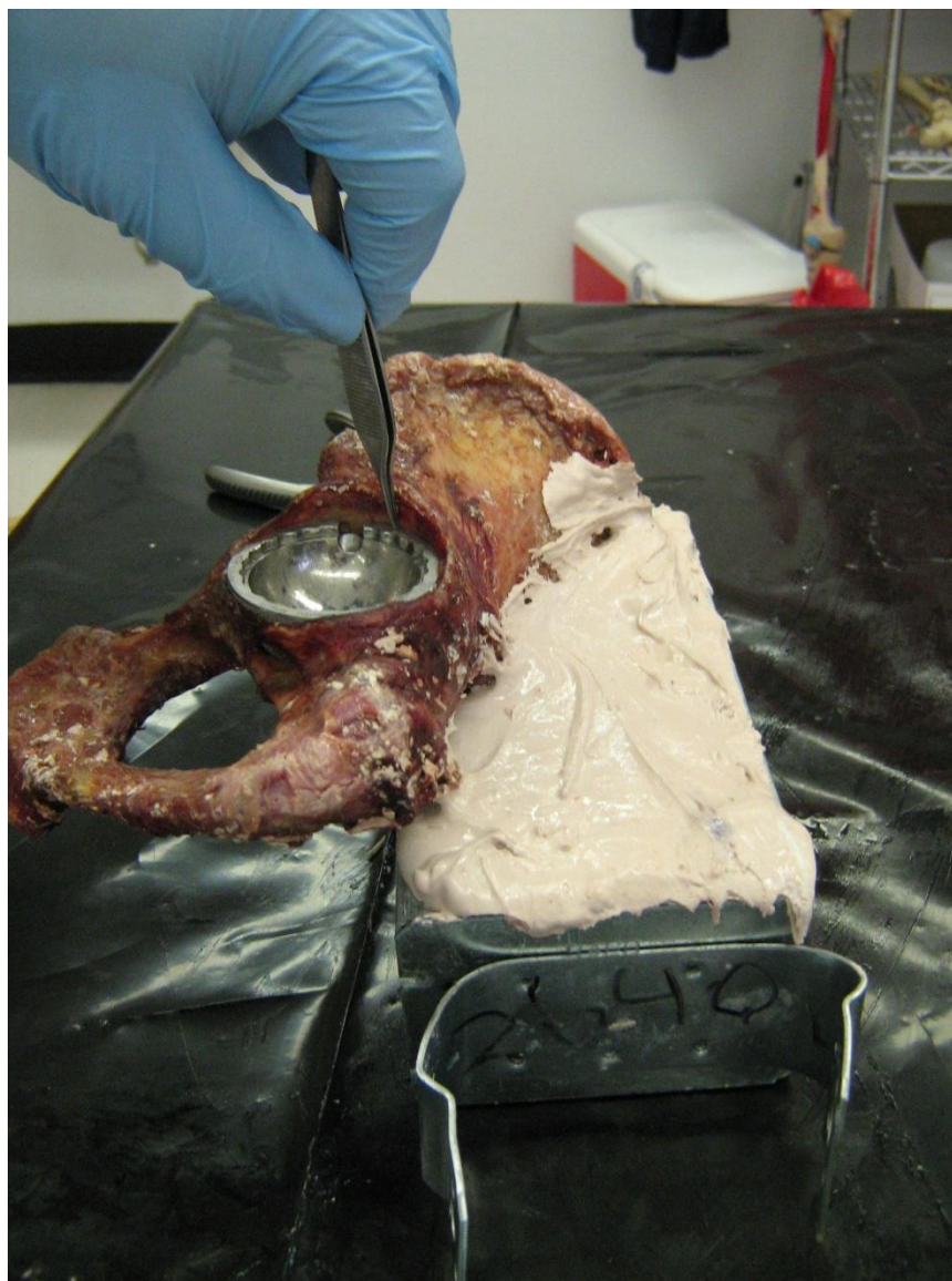
Figure XIX. First control specimen tested. Depuy PINNACLE acetabular cups were press-fit implanted.
