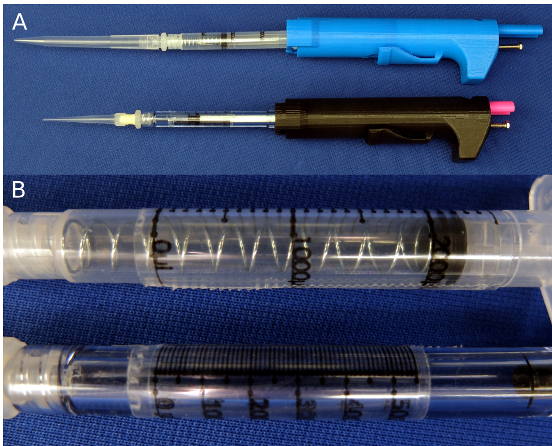
FIGURE 2.8: Photos of assembled pipettes. (A) Two assemblies of the pipette: the 100-1000 \mu\text{L} configuration (above) and the 30-300 \mu\text{L} configuration (below). (B) Close-up photo of the taped on scale for each of the syringes.
