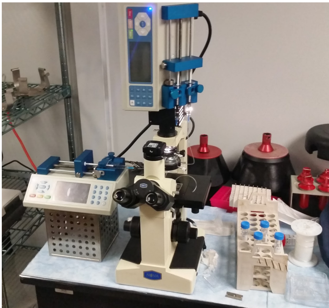
FIGURE 2.14: Encapsulation of cells was performed in a 4°C room with a benchtop inverted microscope.
