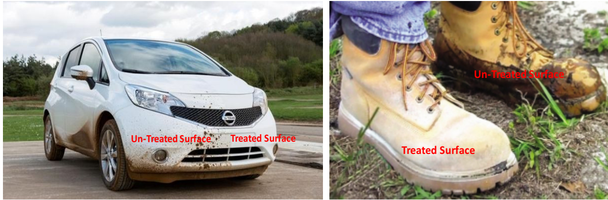
Fig 1.7 – Applications of the super hydrophobic sprays and coatings in daily life. Treated surface represents the spray coating in effect and the un-treated surface is the default surface.
