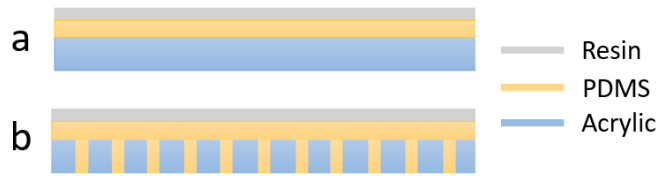
Figure 10. a) Conventional design of constraint surface. b) Air-diffusion-channel design of constraint Surface.
