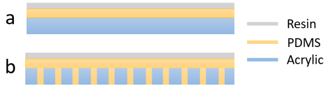
Figure 10. a) Conventional design of constraint surface. b) Air-diffusion-channel design of constraint Surface.
