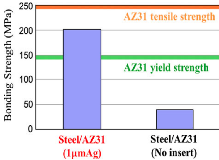
Figure 4. Bonding strengths of steel/AZ31 joints with and without Ag insertion [8].
