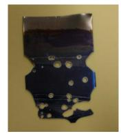
Figure 17 – Ti foil after RBA run
