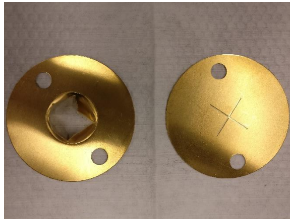
Figure 3 : Prescored soft brass (grade 260) diaphragms used in the UIC-HPST.
