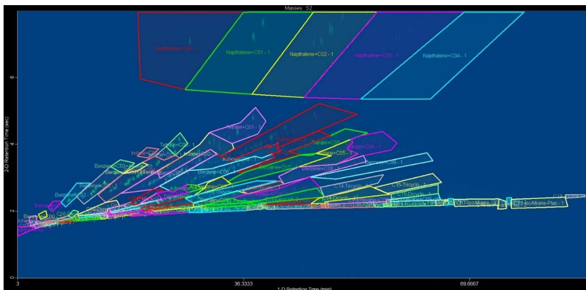
Figure 54 : Two dimensional chromatogram from GCxGC analysis of F-24 illustrating the different classification regions.
