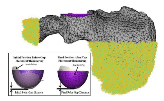
Fig. 5. Finite element model of the hemi-pelvis with constraints at the pubic symphysis and the sacro-iliac
