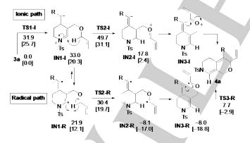
**Scheme 4.** Relative free energies in toluene solution and in the gas phase (in bracket) are in kcal/mol.
