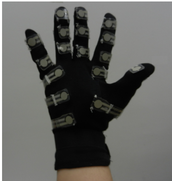
Figure 2. The sensory glove developed in-house
