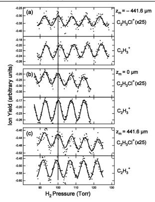
FIG. 3. Modulation data for the parent ion and the C<sub>2</sub>H<sub>3</sub> fragment, measured at (a)  $z_m = -441.6 \ \mu m$ , (b)  $z_m = 0$ , and (c)  $z_m = +441.6 \ \mu m$ . The pairs of modulation curves are shifted horizontally so that the parent ion signals are all in phase. The solid curves are least squares sinusoidal fits to the data, and the vertical dotted line is drawn to guide the eye.
