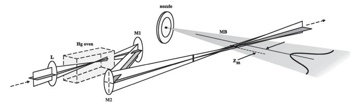
FIG. 2. Schematic drawing of the apparatus. The 532 nm visible laser is focused by a lens L (f = 30.5 cm) into a mercury oven. Mirrors M1 (f = -5.1 cm) and M2 (f = 7.6 cm) are mounted inside the  $H_2$  phase tuning cell (not shown). The two astigmatic foci are separated by 4.6 mm.
