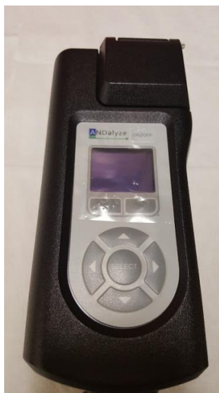
Figure 3: ANDalyze handheld fluorimeter (Model AND1000).
