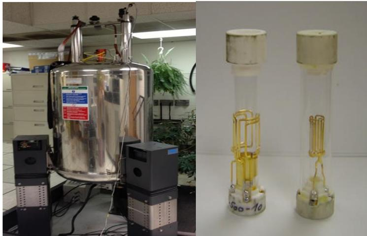
Figure 14: (a) Bruker 500 MHz (11.7 T) micro-imaging facility, (b) Proton and proton/sodium double tuned 5mm RF coil.
