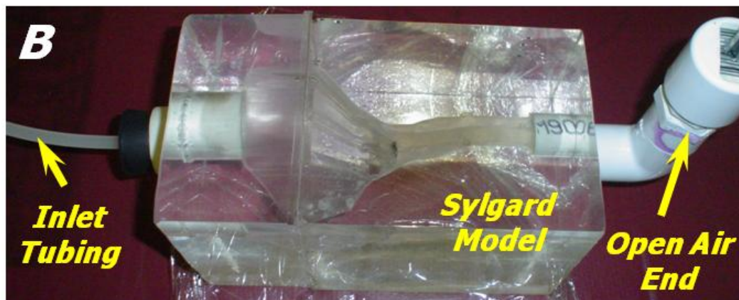
Figure 4.8. Velocity measurements with MRI scanner: A. General setup inside for MRI measurement. B. CM model used in the MRI test.
