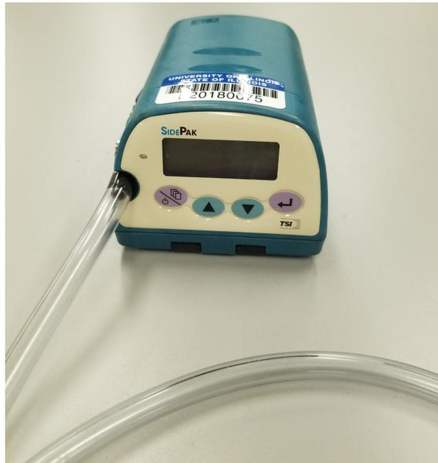
Figure 5: SidePak™ AM510 Personal Aerosol Monitor
