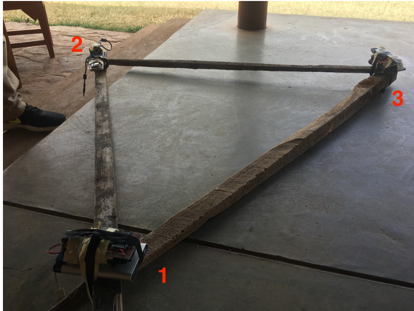
Figure 16: The picture shows the wood structure that has been built to test the GPS module. Three collar units have been attached at the three corners of the structure in order to have them at a distance of 1.2m from each other.
