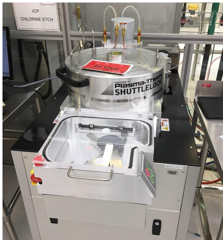
Figure 31. Plasma-Therm ICP Chlorine Etch System. Etching system which is used to etch the \text{Al}_2\text{O}_3 layer.
