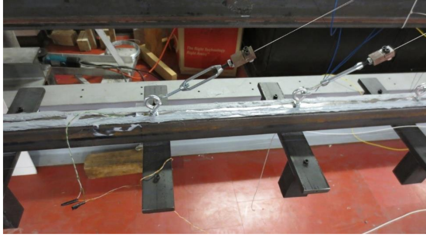
Figure 10. Steel plates and close up view of the adhered distributed fiber
