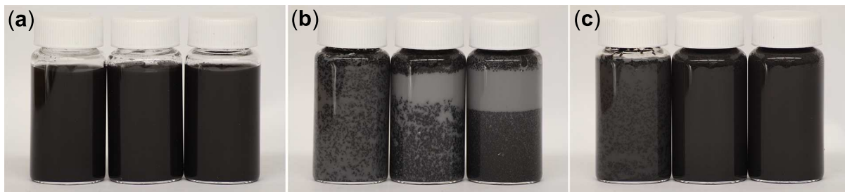
Figure 10. (a) xGnP-water suspensions in 20 mL glass vials with varying concentration of \text{NH}_3(\text{aq}) (left vial 0 wt.%, middle vial 1.0 wt.%, right vial 7.7 wt.% \text{NH}_3(\text{aq}) ). (b) The vials from a with 1 g of a 42 wt.% PE dispersion in water added to each. (c) The vials from b after 60 min of bath sonication. Note the apparent stability of the dispersion in the rightmost vial.
