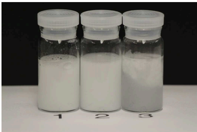
Figure 8. 15 mL vials all containing 0.12 g of polyethylene copolymer in 10 g of water. Vial 2 also contains \sim 1 g of ammonium hydroxide, while vial 3 also contains 1.6 g of acetic acid.
