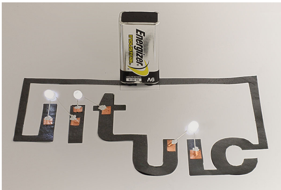
Figure D6. A simple circuit was fabricated to display the collaboration between the Italian Institute of Technology (IIT) and the University of Illinois at Chicago (UIC). The circuit was designed such that the three LED lights would bridge the circuit forming a connection at the three i's in the logos. The LED's were affixed with adhesive copper tape, with a spot of silver paint to ensure good contact. The paper was sprayed with Strem 25 \mu\text{m} (S-25) MLG particles in a 50 wt. % blend with the CuPC paint solids. The electrical circuit is closed once the battery is placed upside down on the two conductive paper leads, and the i's are "dotted" with a bright white light.
