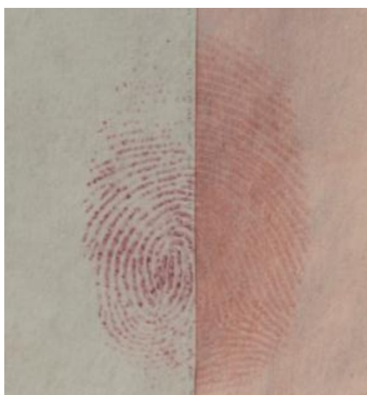
Figure 6. Image of a latent fingerprint developed with ninhydrin (left) and Oil Red O (right).
