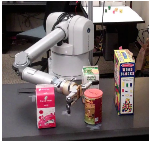
Figure 2: Barrett Whole Arm Manipulator (BarrettWAM).
