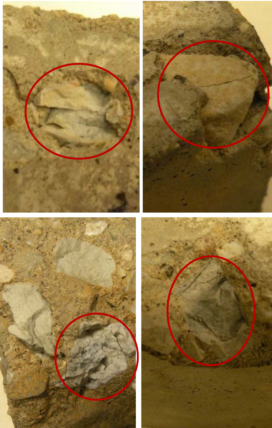
Figure 9-4. Typical aggregate popout in Freeze/thaw specimens
