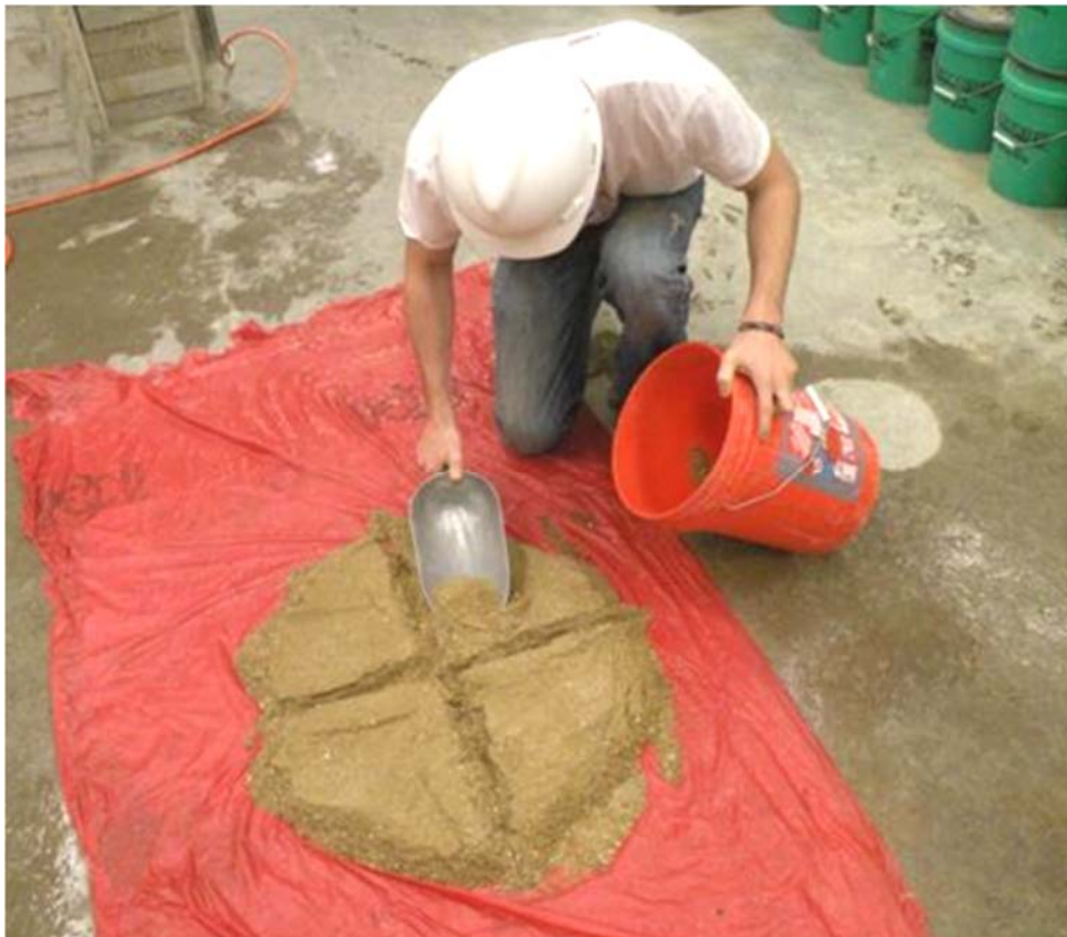
Figure 3-3. Quartering of fine aggregate for gradation sampling.
