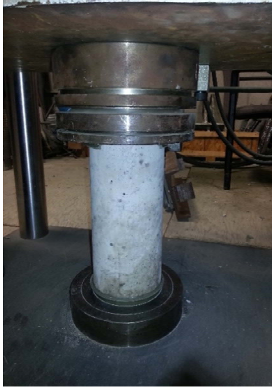
Figure 5-2. Test configuration for the compressive strength per ASTM C39
