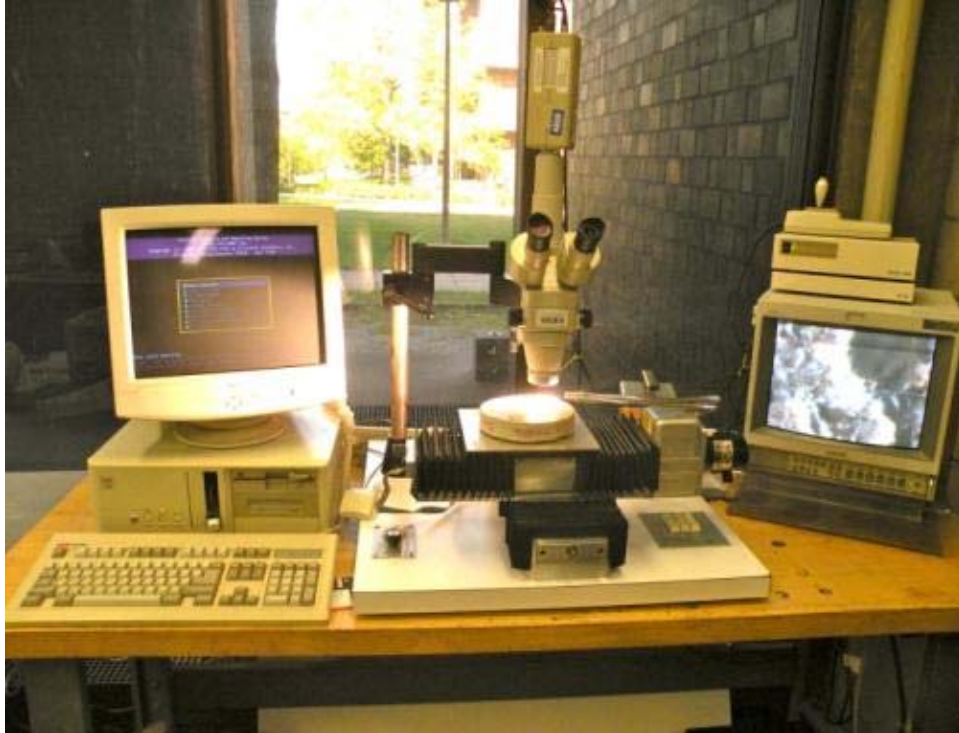
Figure 5-5. Microscopic determination of air void system parameters (ASTM C457).
