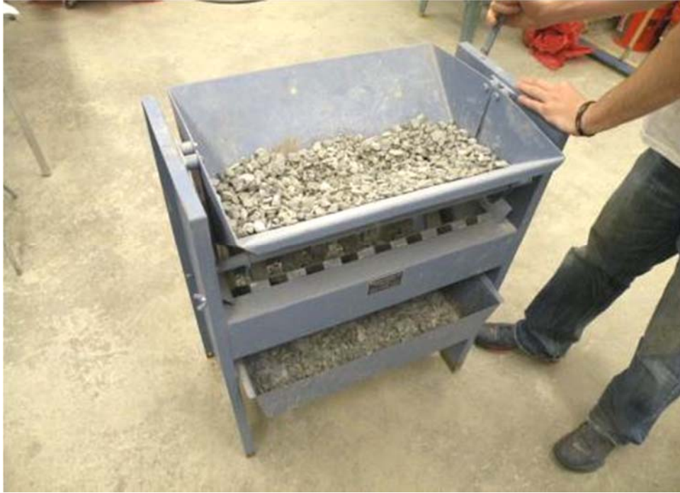
Figure 3-2. Mechanical splitting device for coarse aggregate gradation sampling.
