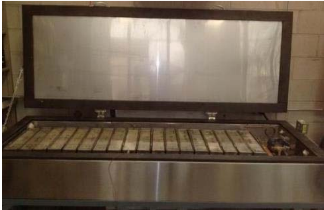
Figure 5-6. Freeze/thaw test cabinet, ASTM C666, procedure A.
