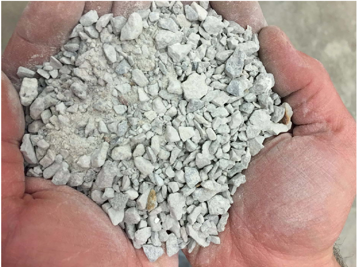
Figure 2-1. Excess crushed limestone usable for concrete
