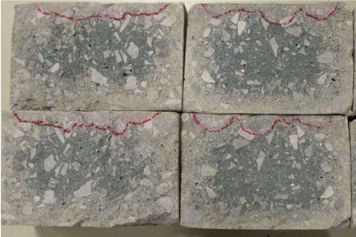
Figure 5-12. Depth of water penetration in split DIN 1048 specimens
