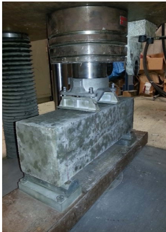
Figure 5-3. Test configuration for the flexural strength of concrete per ASTM C78
