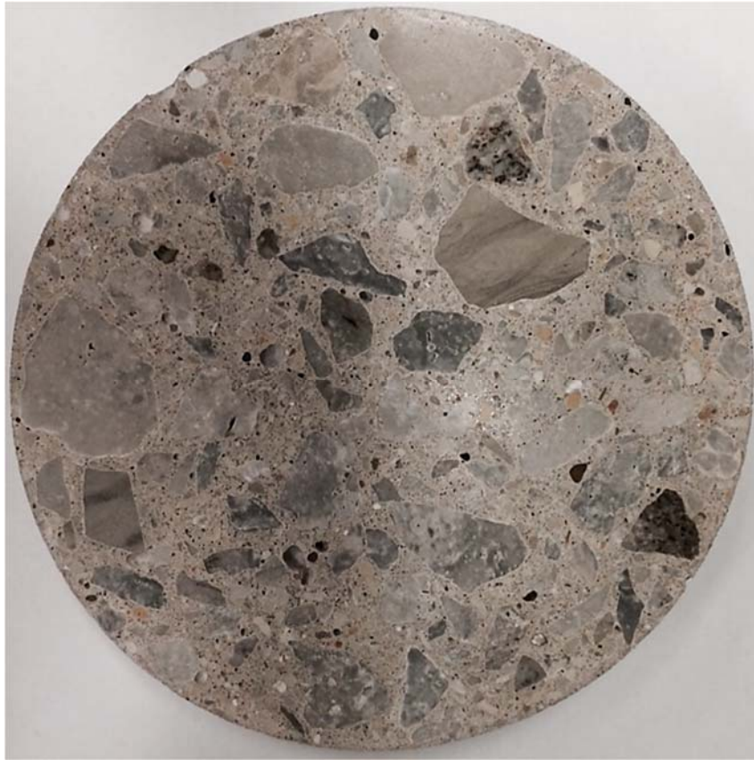
Figure 5-4. Concrete specimen prepared for air void measurement.
