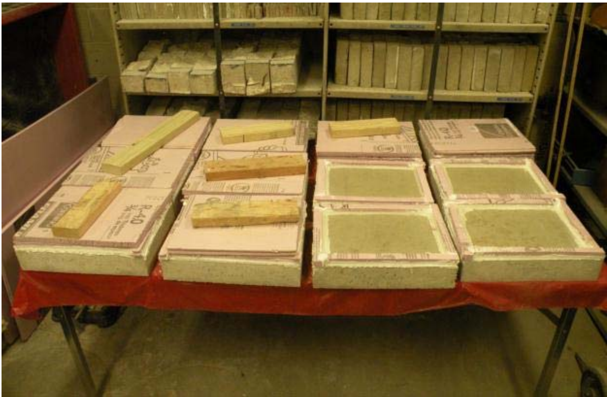
Figure 5-13. Salt ponding test (chloride content across the slab depth).
