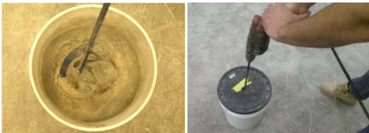
Figure 3-1. Preparing C3 cement by blending C1 cement with fly ash.
