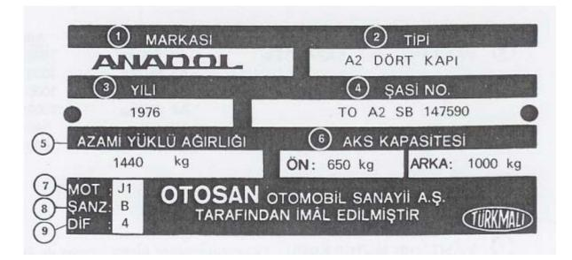
Figure 4.8 Vehicle info plate of an Anadol car, c. 1970s.
