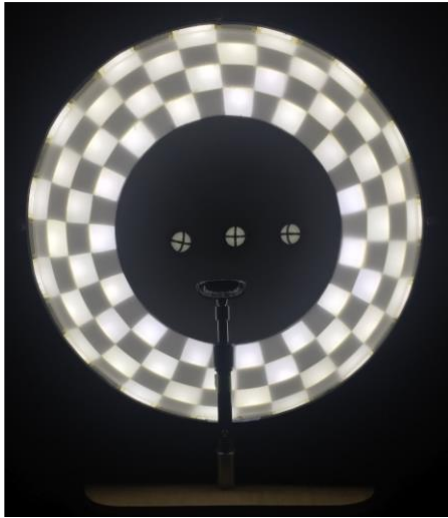
Figure 7. Updated system setup. (A) System set up for human subject recording. The chin rest is incorporated to provide a stable head position during the recording. (B) System set up for animal (rat) experiments. The interchangeable chin rest replaced with a custom designed animal mount; the mount accommodated a heating pad to maintain normal body temperature (37°C). Three-axis manipulator seen in the image was used to lower the recording (looped platinum needle electrode) to the eye. The recording electrode was later replaced by a DTL fiber electrode.
