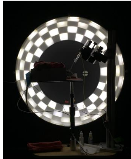
Figure 7. Updated system setup. (A) System set up for human subject recording. The chin rest is incorporated to provide a stable head position during the recording. (B) System set up for animal (rat) experiments. The interchangeable chin rest replaced with a custom designed animal mount; the mount accommodated a heating pad to maintain normal body temperature (37°C). Three-axis manipulator seen in the image was used to lower the recording (looped platinum needle electrode) to the eye. The recording electrode was later replaced by a DTL fiber electrode.
