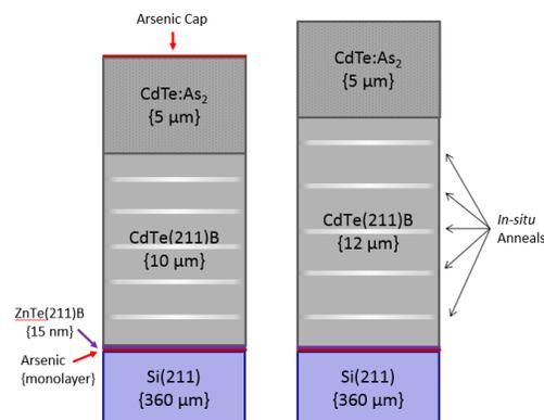
Figure 55: Thick Buffer CdTe:As<sub>2</sub> sample stacks
