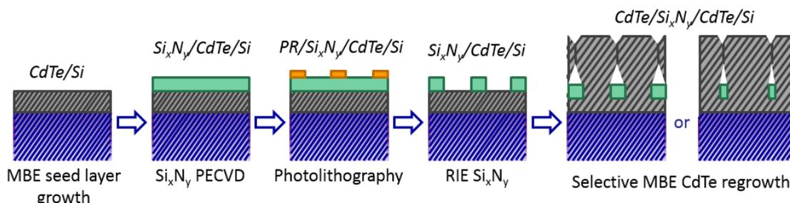
Figure 70: Patterning and growth process diagram for pseudo-*px*-CdTe deposition.
