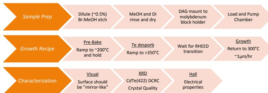
Figure 81: Standard MBE CdTe regrowth process.
