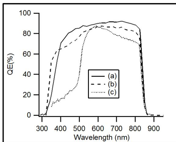
Figure 22: QE measurement showing differences in (a) NREL's best lab cell [53], (b) a 15% cell produced at EPIR measured by NREL, and (c) a sample production cell [53]. [10, 11]
