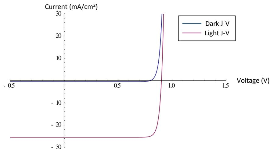
Figure 6: Ideal diode current voltage characteristic with and without illumination.
