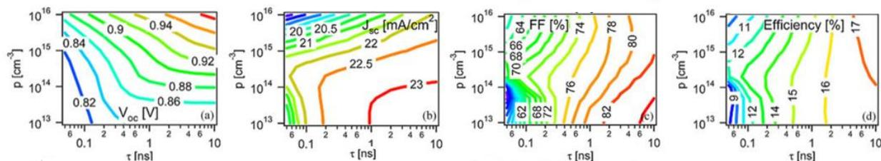
Figure 2:  $V_{oc}$ ,  $J_{sc}$ , FF, and Efficiency (left to right) plotted vs.  $N_A$  ( $p$ ) and lifetime ( $\tau$ ) [17]
