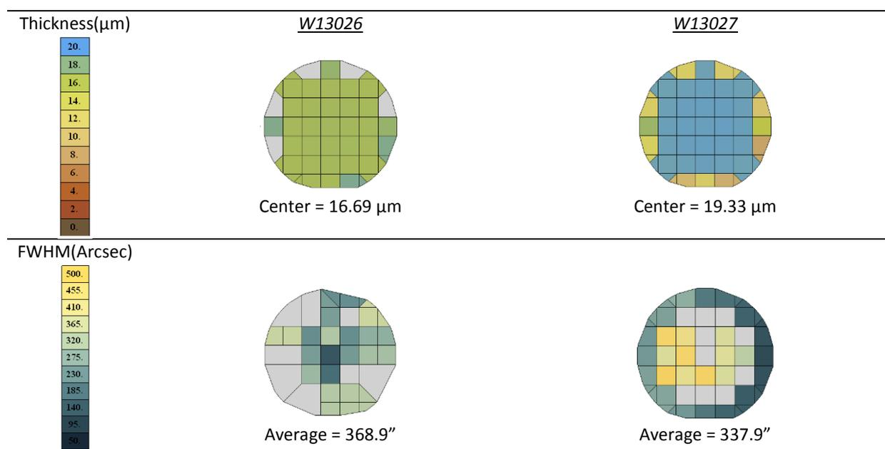
Figure 56: FWHM and Thickness Maps for preliminary arsenic doped CdTe samples
