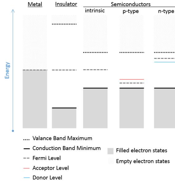
Figure 4 : Simple energy band diagrams for metals, insulators, and semiconductors. A p-n junction is then formed by bringing together an n-type and a p-type material. P-n junctions are one of the most fundamental semiconductor systems and have been exhaustively characterized over the last many decades [26, 27].
