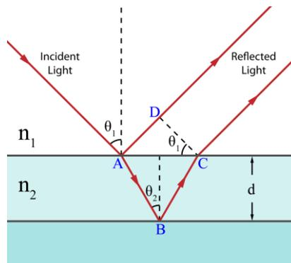
Figure 14: Thin film interference diagram [45]
