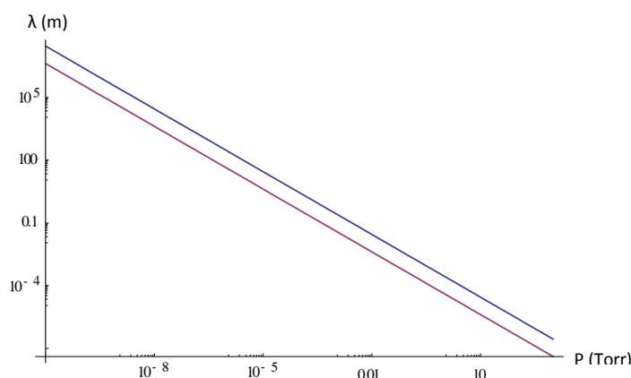
Figure 27: Mean Free Path of Cd or Te<sub>2</sub> in room temperature ambient as function of pressure.
