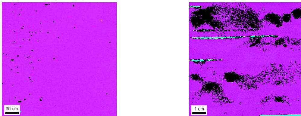
Figure 78: EBSD maps for mostly sx-CdTe portion of sample W13022(-20,20).
