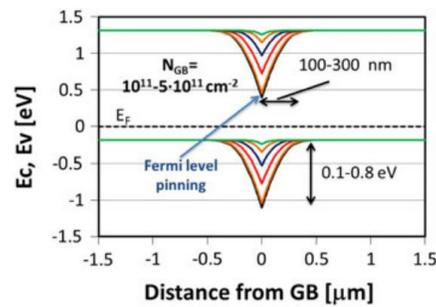
Figure 64: Local band bending modeled around Cl enhanced grain boundary with vary levels of Cl concentration [25].
