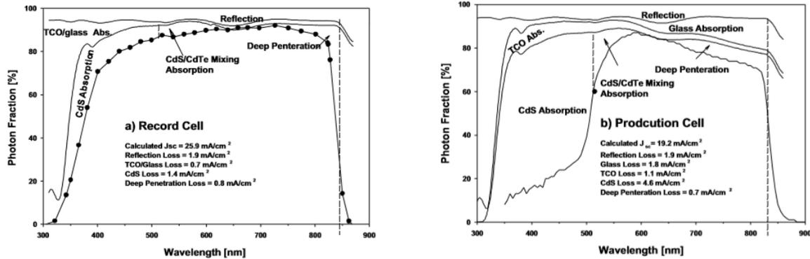
Figure 17: Quantum Efficiency of the NREL 16.7% Record device (left) and a typical production cell (right) as found in the paper “Quantification of losses in thin-film CdS/CdTe solar cells” by Demstu and Sites [53].
