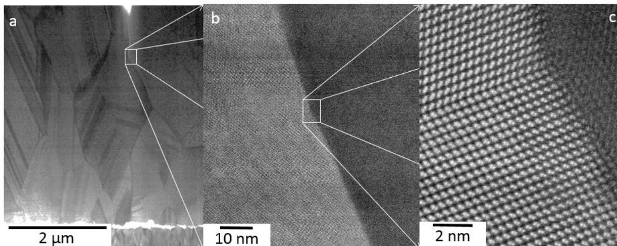
Figure 24: STEM images showing several types of defects in polycrystalline CdTe material deposited by CSS.
