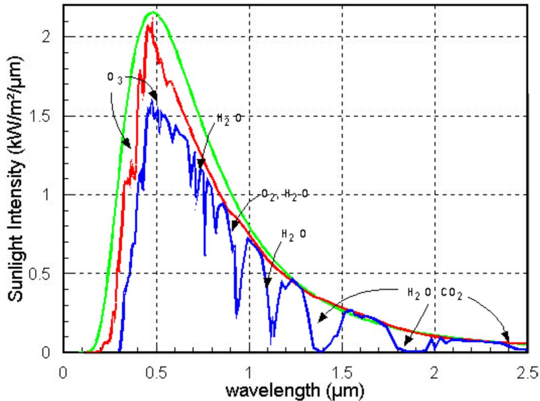
Figure 8: Green = Blackbody at 6000K; Red = AM0 spectrum; Blue = AM1.5 spectrum with absorption notes. [32]
