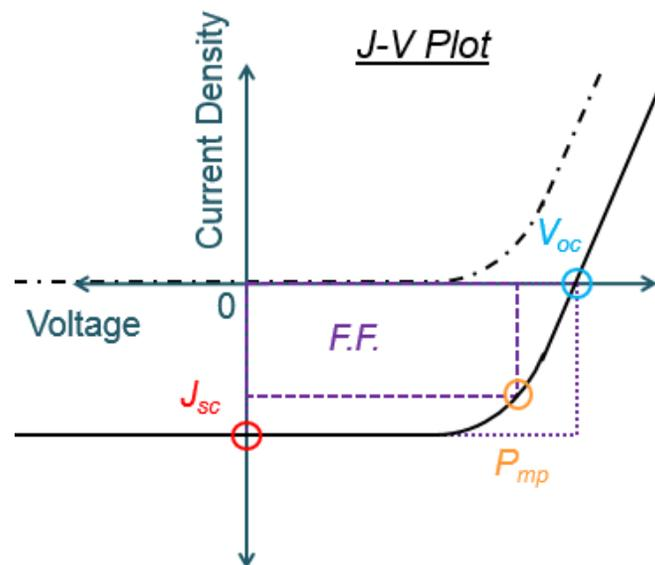
Figure 7: Current voltage characteristic for an illuminated p-n junction with standard device metrics indicated.
