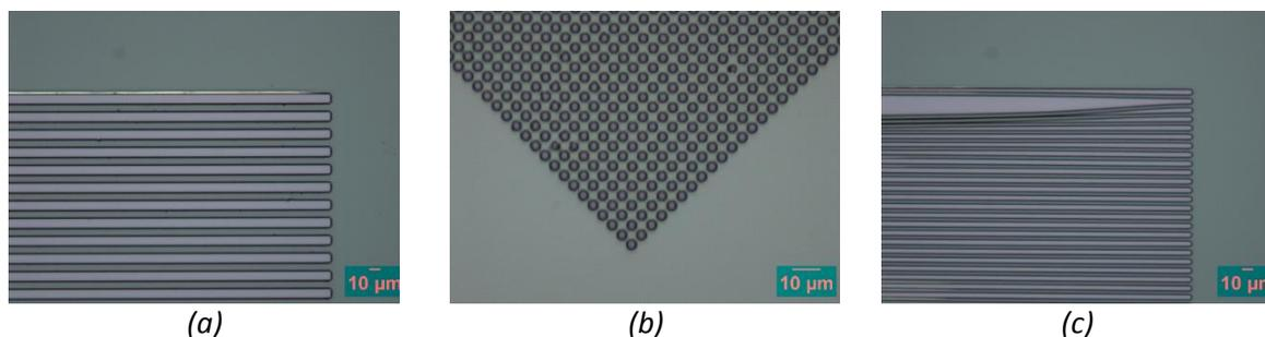
Figure 74 : “Bar” features separated by  $8\ \mu\text{m}$  (a). Rotated  $5\ \mu\text{m}$  pitch with  $3\ \mu\text{m}$  features (b). “Bar” features separated by  $4\ \mu\text{m}$  showing undesired feature lift-off.
