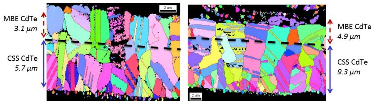
Figure 69: Cross-sectional EBSD of MBE regrown polycrystalline CdTe; R1746-6:CTP6 (left); R1753-4:CTP6 (right)
