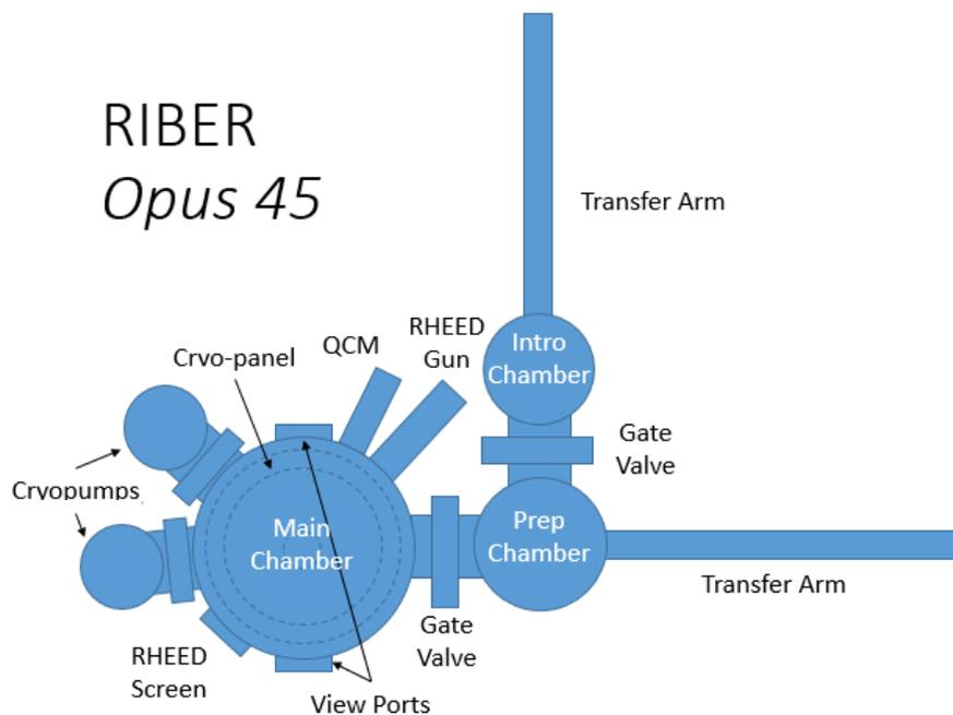
Figure 29: Top down view of the Opus 45 MBE system used for this thesis.
