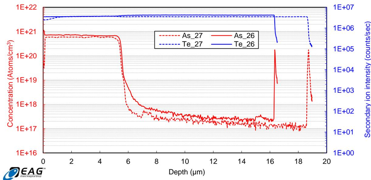
Figure 57: SIMS profiles for preliminary arsenic incorporated samples.
