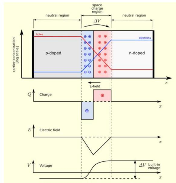
Figure 5: Basic p-n junction diagram. [31]
