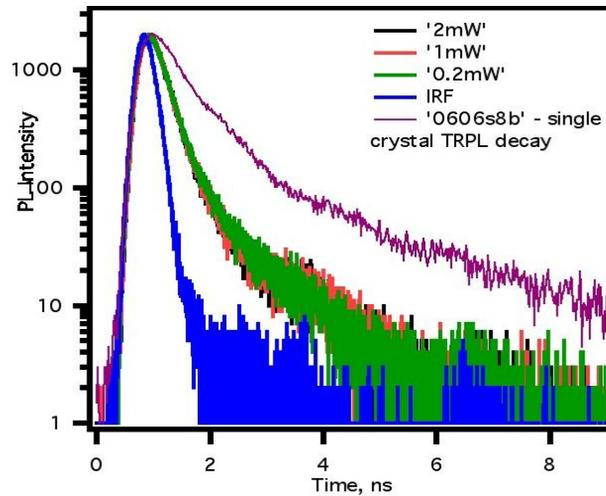
Figure 41: TRPL curves for a single crystal CdTe on Si sample at three different excitation powers (Black, Red, Green) compared with a bulk CdTe sample (purple), and the system response (Blue).
