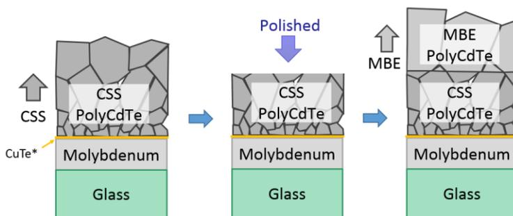
Figure 66: MBE px-CdTe regrowth sample stack and processing progression. \*Only certain samples have a CuTe layer
