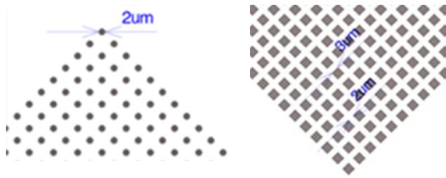
Figure 73: 2  $\mu\text{m}$  round features (left); 3  $\mu\text{m}$  square features (right)
