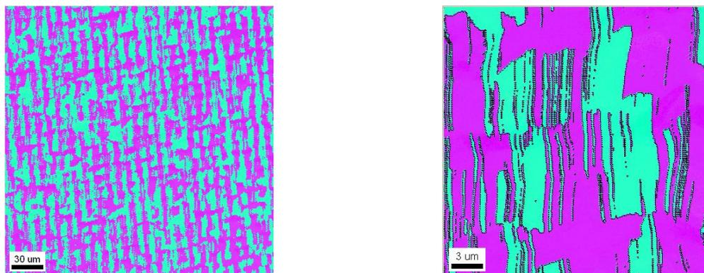
Figure 79: EBSD maps for pseudo-px-CdTe portion of sample W13022(-20,20).
