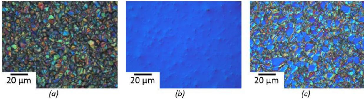
Figure 68: CSS CdTe surface prior to polishing (a), CSS CdTe surface after polishing (b), and MBE CdTe surface after regrowth (c)
