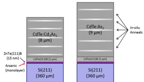
Figure 58: CdTe:Cd<sub>3</sub>As<sub>2</sub> vs. CdTe:As<sub>2</sub> sample stacks
