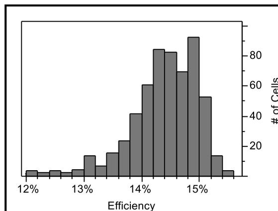
Figure 23: Histogram of devices efficiency for the hundreds of cells produced at EPIR between December 2010 and June 2011 with a buffer layer [10, 11].
