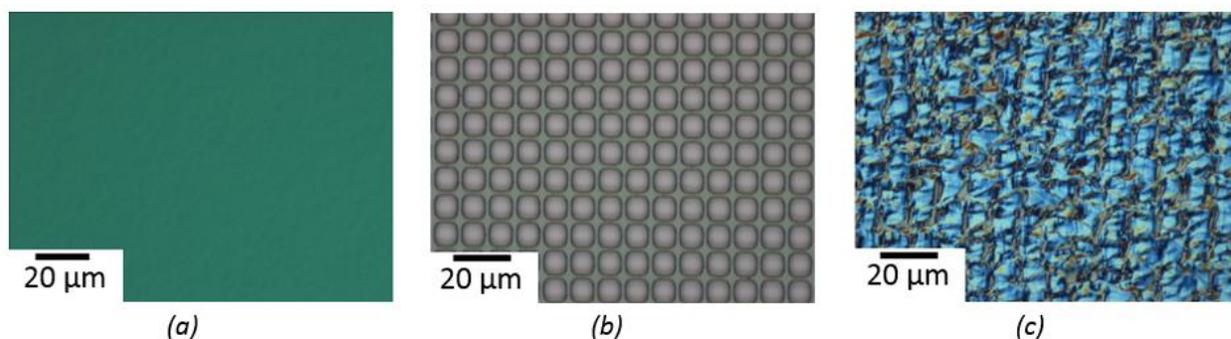
Figure 75: Optical images of single crystal CdTe seed layer surface (a) ; Patterned photoresist on SiN (b) ; and pseudo-px-CdTe deposited by MBE.
