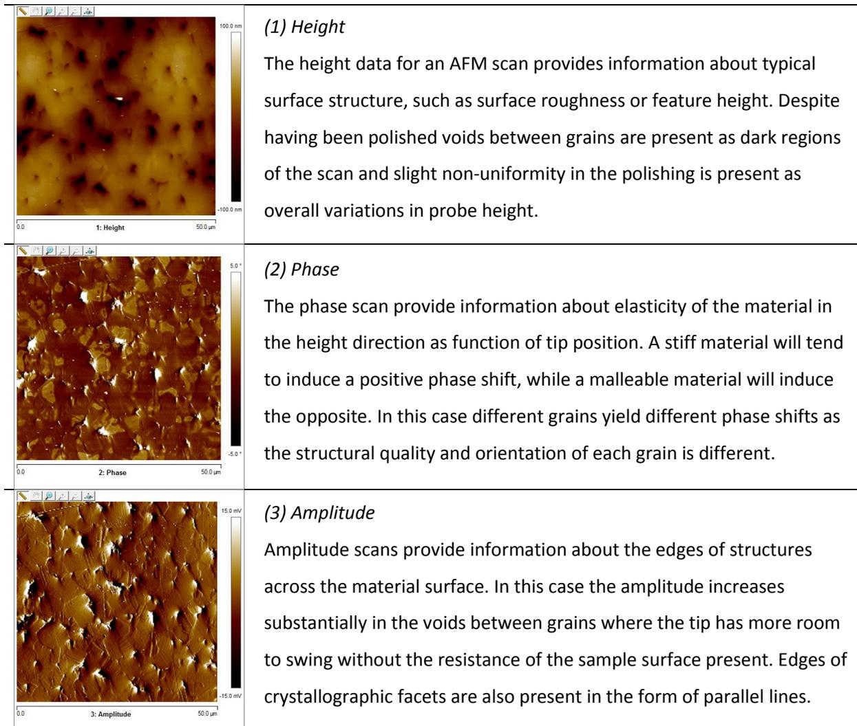
Figure 16: Height, Phase, and Amplitude data for 50x50 $\mu\text{m}$  AFM scan of sample CSS px-CdTe sample R1753-3 after polishing.
