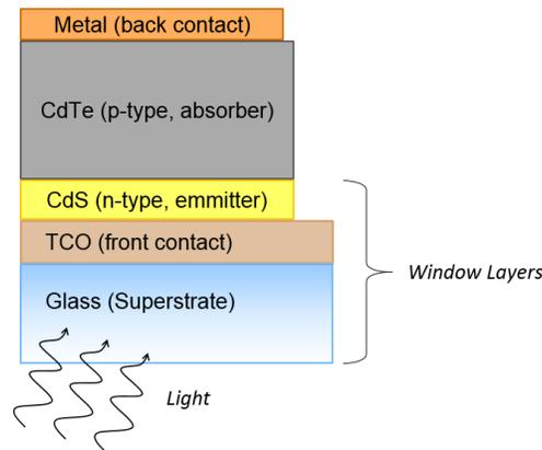
Figure 1: Standard thin film CdTe solar photovoltaic device structure
