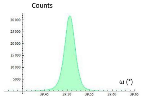
Figure 39: Example CdTe XRD 422 DCRC peak. FWHM=0.024°=86"
