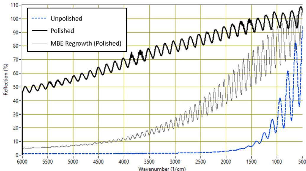
Figure 67: FTIR spectrum unpolished (130710-4-d), pre-MBE polished (C130710-2-a), and post-MBE regrowth on the polished substrate (C130710-2-a:W13018).
