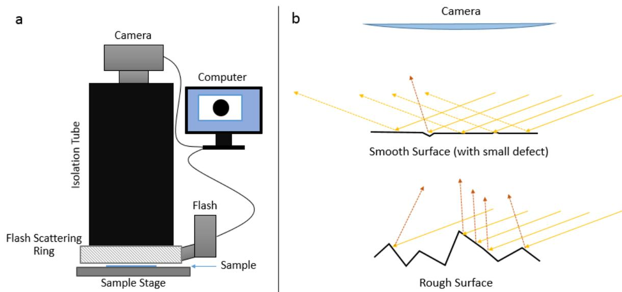
Figure 36: (a) Optical Scattering set-up (b) Schematic diagram of the basic principle of optical scattering. The Smooth surface scatters only a small portion of the incident illumination to the camera, while the rough surface scatters a significant portion of the incident light back to the camera.
