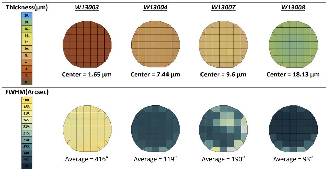
Figure 46 : FTIR Thickness and XRD <422> DCRC FWHM wafer maps
