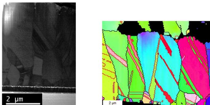
Figure 62: Cross sectional low magnification STEM ABF image (left, [63]) and EBSD [96] showing smaller grains at nucleation interface (bottom of the images) compared to the larger size.
