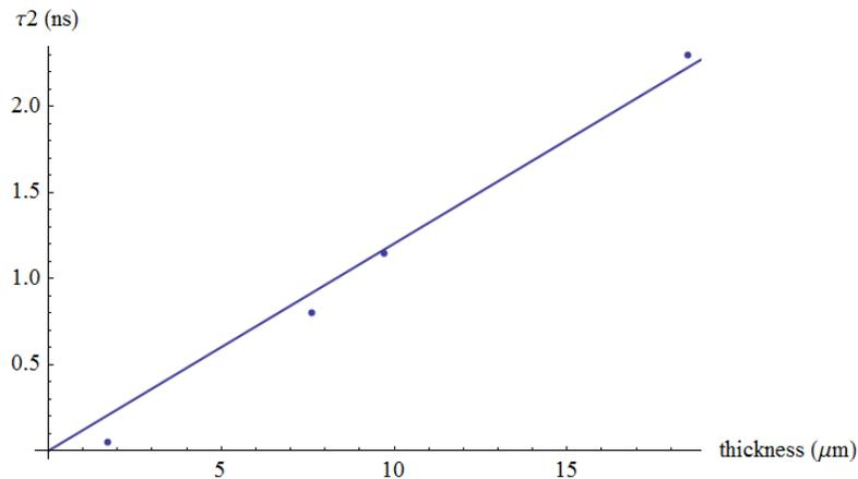
Figure 48: Carrier recombination Lifetime plotted vs. CdTe layer thickness.
