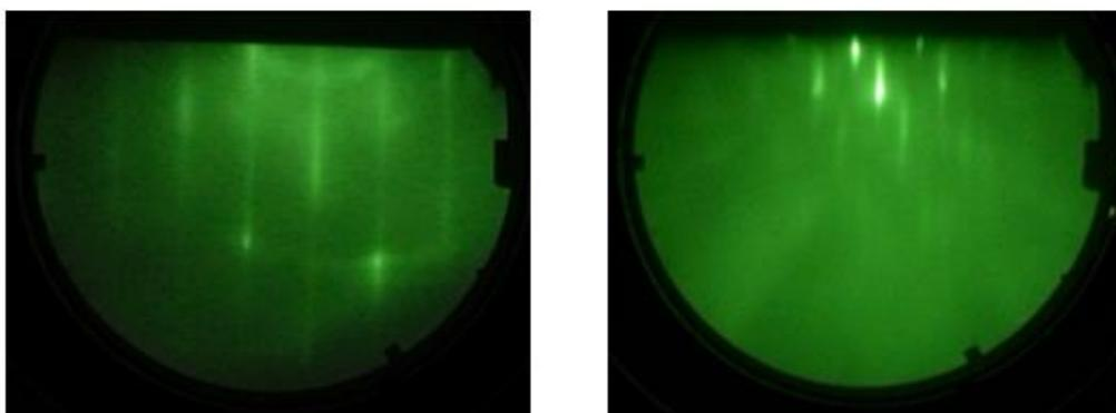
Figure 40: RHEED Patterns along the (110) axis for Si(211) {left} after the high temperature oxide desorb, and CdTe(211) {right} after  $\sim 10 \mu\text{m}$  growth.
