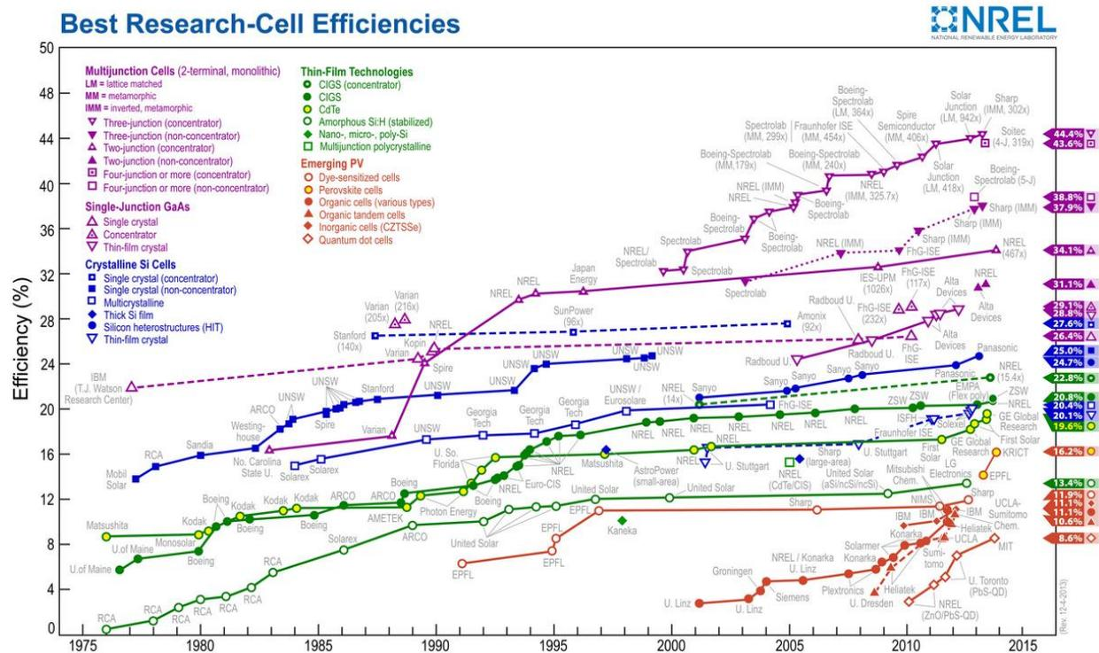
Figure 10: NREL Best Research-Cell Efficiencies over time plot [13].
