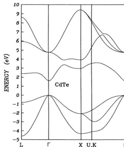
Figure 3: CdTe Band Structure showing direct band-gap at the gamma point. [30]
