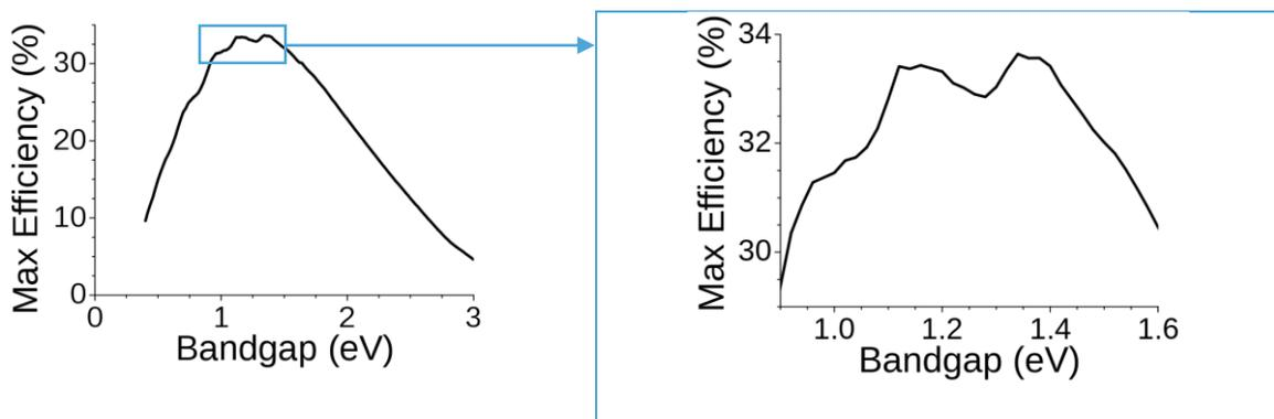
Figure 9: Left = Shockley-Queisser limit for broad range of band gaps. Right = Zoomed in between 1 and 1.6 eV band gaps. [33]
