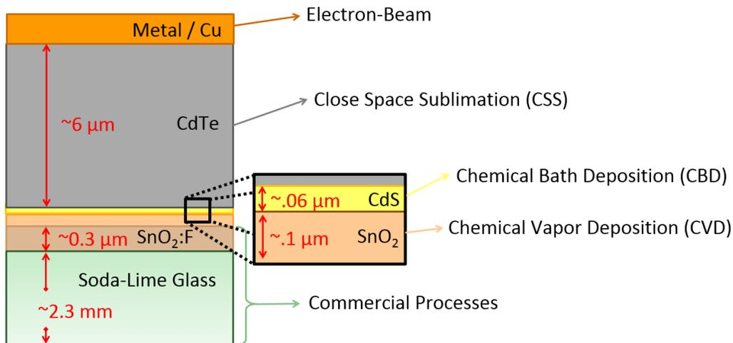
Figure 21: This is a schematic diagram of the device structure, typical layer thicknesses, and individual layer fabrication processes associated with each layer for the thin film CdTe solar cells in this thesis.
