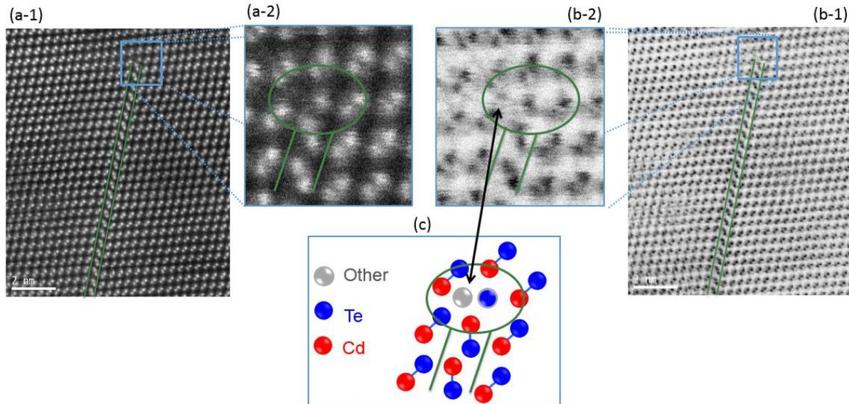
Figure 19: HAADF image of CdTe micro-twin terminated by a dislocation (a-1), further magnified in (a-2). ABF image of the same micro-twin terminated by a dislocation (b-1), further magnified in (b-2). A model basic of the system (c) identifying the presence of a lighter element within the dislocation as seen by the ABF image.
