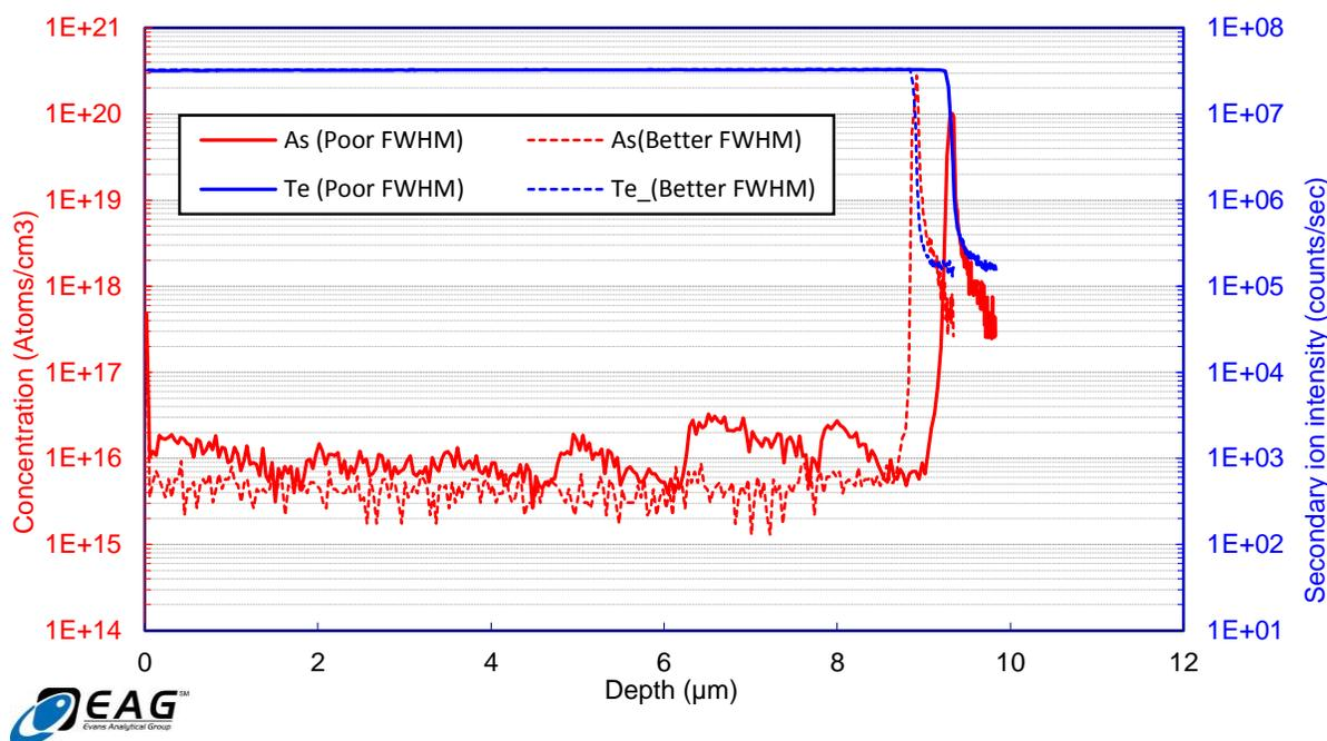
Figure 61: SIMS for two regions of sample W13032, one with good crystal quality and the other with poor crystal quality.
