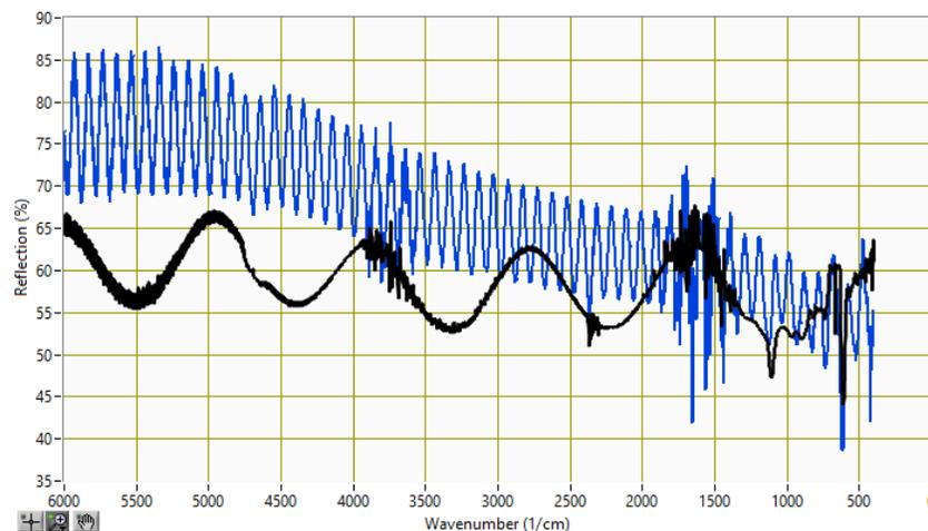
Figure 38: FTIR single point measurement for samples W13003 (Black, 1.6  $\mu\text{m}$ ) and W13008 (Blue, 17.5  $\mu\text{m}$ )
