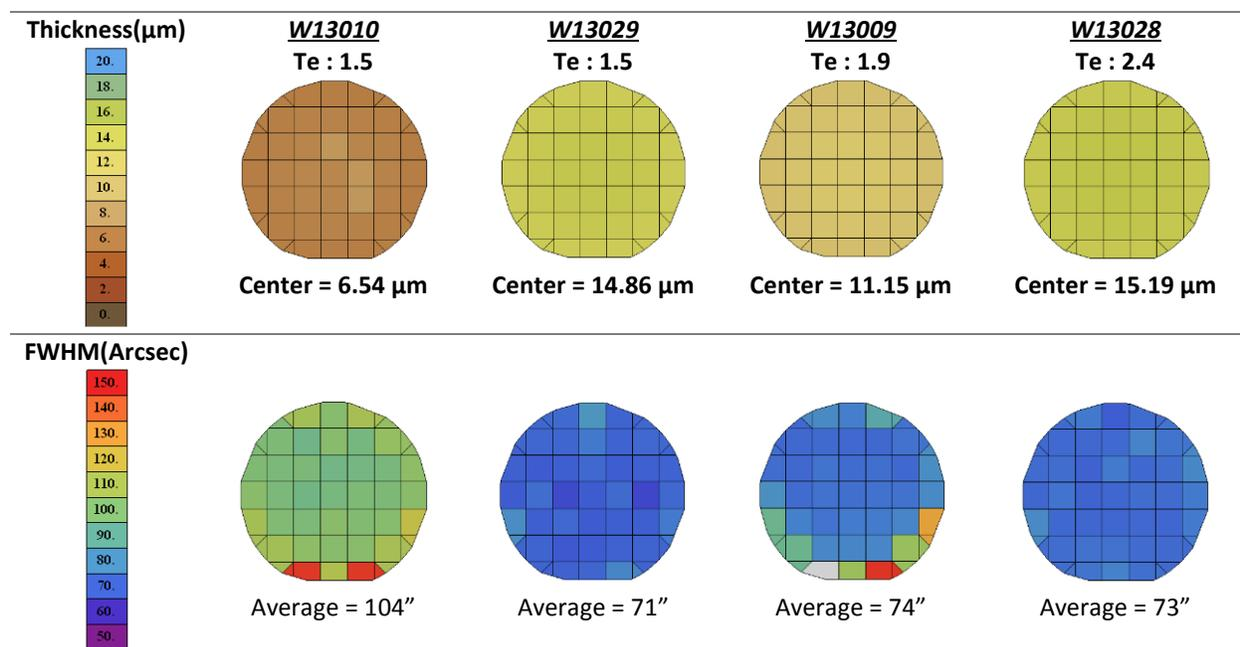
Figure 51: Thickness and FWHM Maps for Te overpressure samples.
