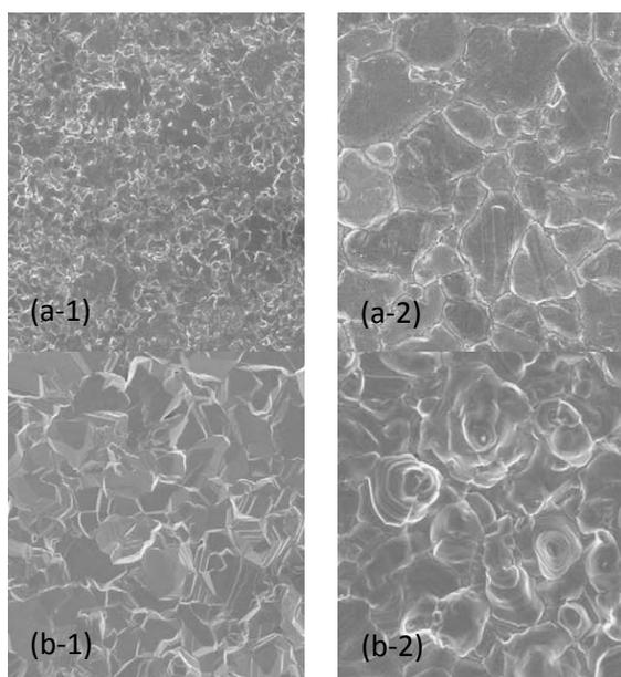
Figure 63: SEM images at the same magnification of the surfaces CdTe deposited by Evaporation (a) and CSS (b) before (1) and after (2)  $\text{CdCl}_2$  treatment [98].
