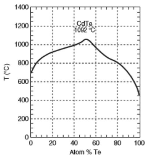
Figure 11: CdTe phase diagram. Melting point vs. Te%. [35, 37]
