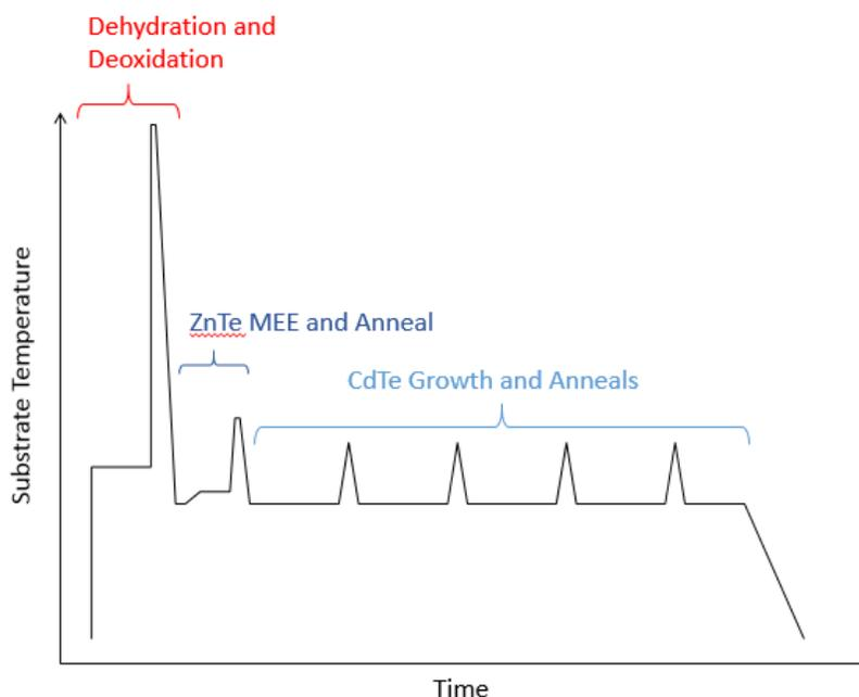
Figure 35: Typical substrate temperature progress for single crystal CdTe on Si growth.
