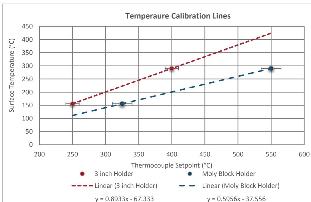
Figure 32: Opus sample holder surface to set-point temperature calibration lines.
