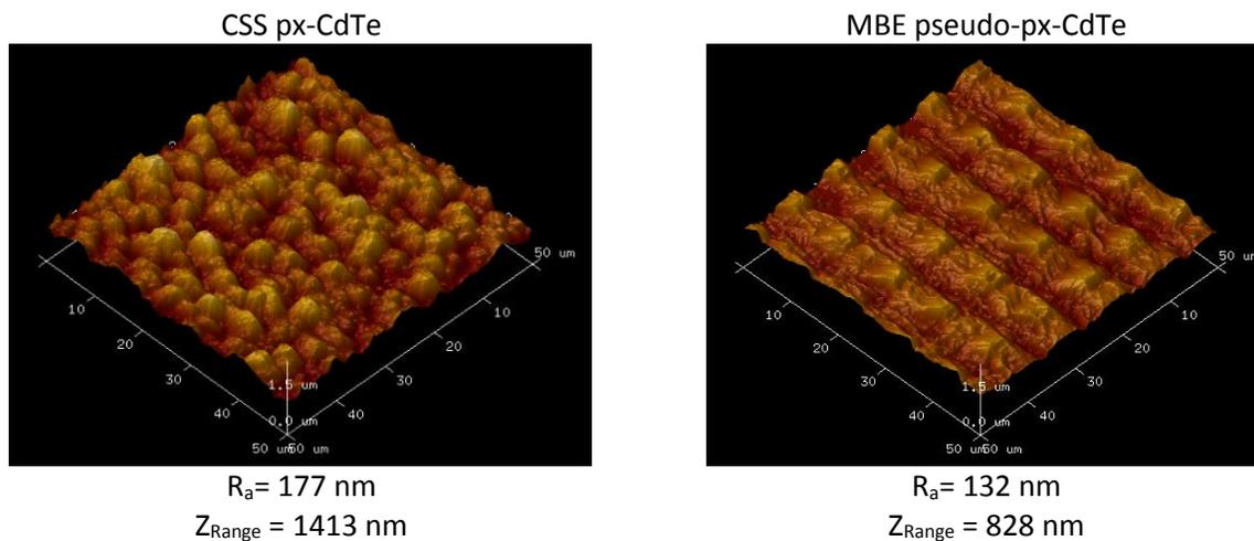
Figure 80: AFM comparing surface morphology of px-CdTe and MBE pseudo-px-CdTe (sample W13023)
