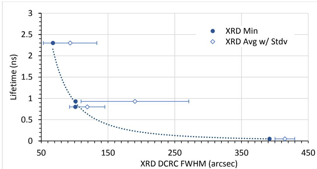
Figure 47: Plot comparing crystal quality (FWHM) to recombination rate ( $\tau_2$ ).
