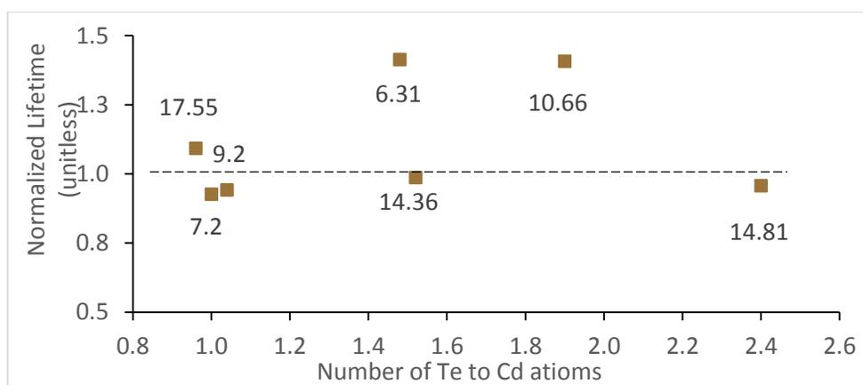
Figure 53: Normalized Lifetime vs. Te ratio. Point labels are CdTe thickness in  $\mu\text{m}$
