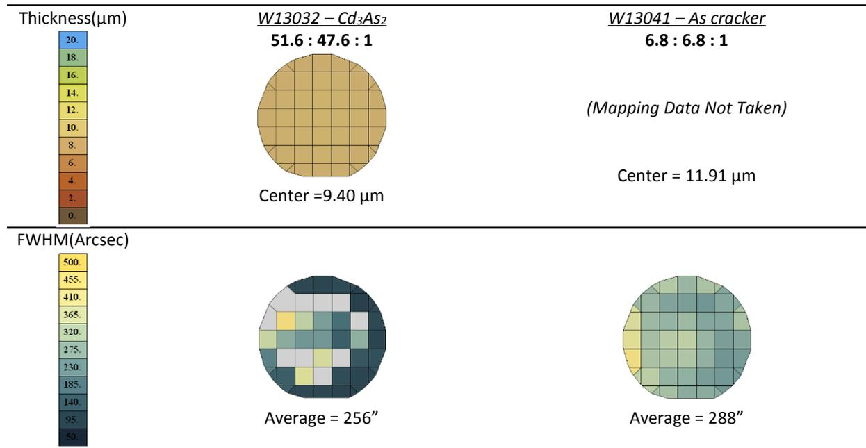
Figure 59: FWHM and Thickness Maps for preliminary arsenic doped CdTe samples
