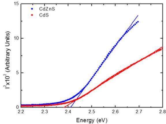
Figure 13:  $(\alpha \cdot hv)^2$  vs.  $hv$  plot for CdS and low Zn concentration CdZnS with linear portion fitted, showing the slightly increased band gap of CdZnS.
