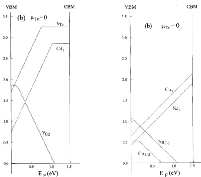
Figure 50: Formation energies as a function of Fermi Level in the Te-rich limit [88].
