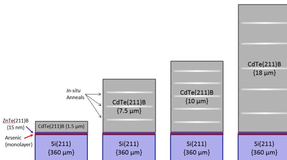
Figure 45: Thickness variation baseline sample stacks.
