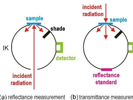
Figure 15: Spectrophotometer integrating sphere diagram [47]
