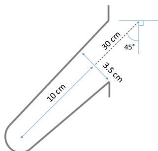
Figure 30: Cross section of PBN source crucible for effusion cells on Opus
