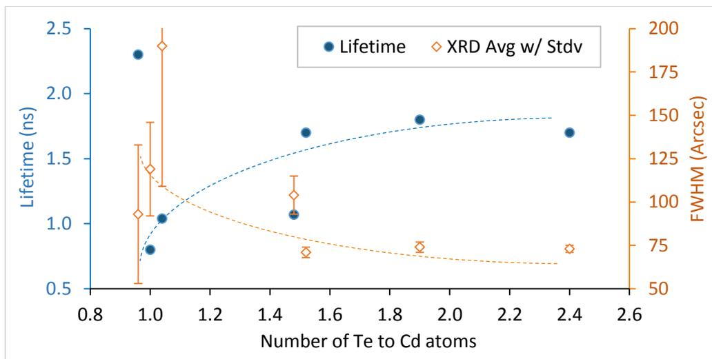
Figure 52: Lifetime and FWHM vs. Te ratio. Trend line added to guide the eye. Points with identical Te ratio values scattered to avoid misreading associated points.
