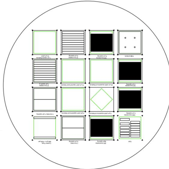
Figure 71: Full 3'' shadow mask design for pseudo-px-CdTe
