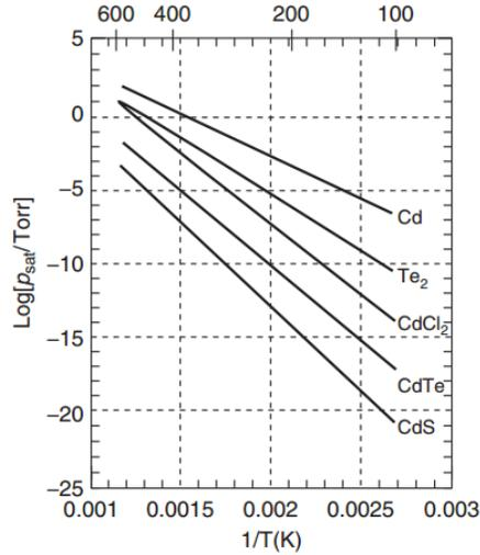
Figure 28: Vapor Pressure vs. Temperature of some source materials [35].
