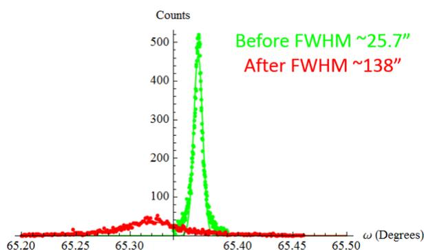
Figure 82: Before (Green) and after (Red) XRD DCRC scans for sample W13022 CdTe(110) re-growth
