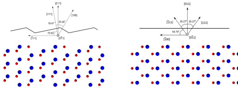
Figure 83: Comparison of CdTe(211) {left} and CdTe(011) {right} surface with (111) and (100) growth orientations identified
