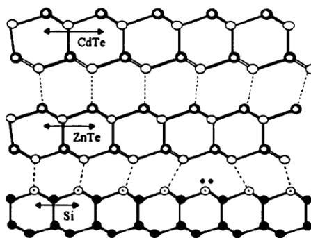
Figure 34: Si, ZnTe, CdTe (111) orientation lattice size [75]
