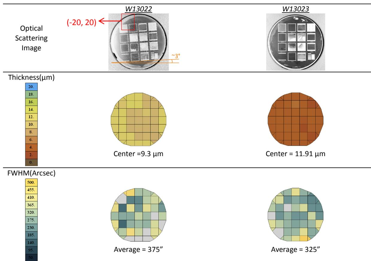
Figure 76: Pseudo-px-CdTe Samples Optical Scattering, FWHM and Thickness Mapping
