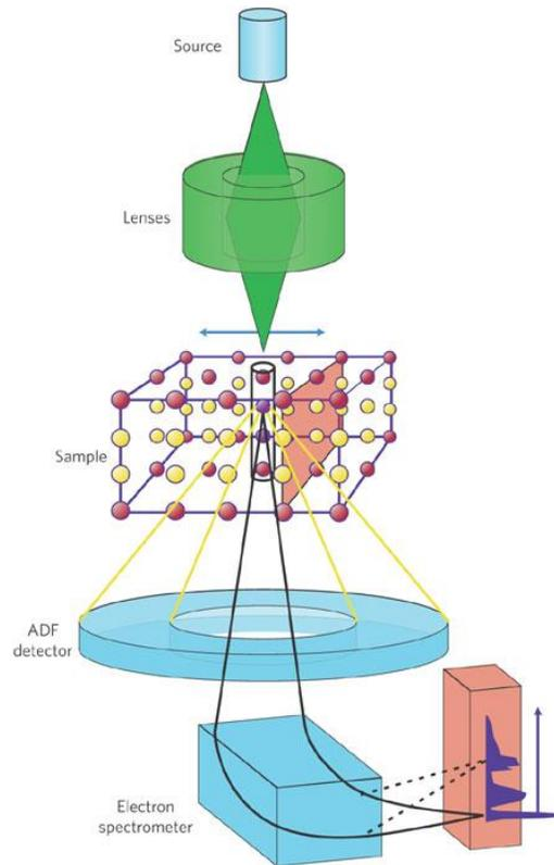
Figure 18: Schematic Diagram of STEM system [56].
