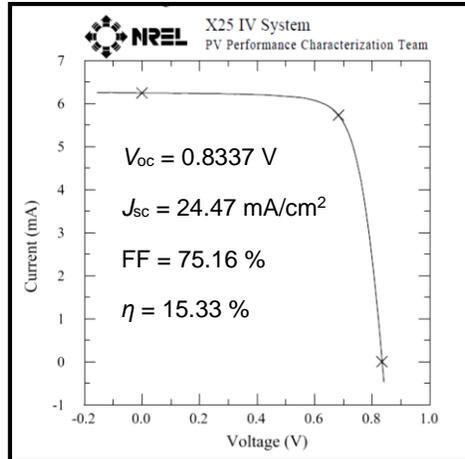
Figure 20: NREL-verified J-V characteristic and extracted device parameters for 15.3% champion thin film CdTe device.
