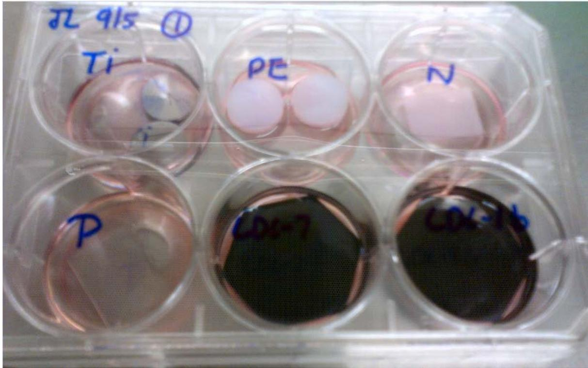
**Figure 9: Extraction of CDC Tile Specimen**
