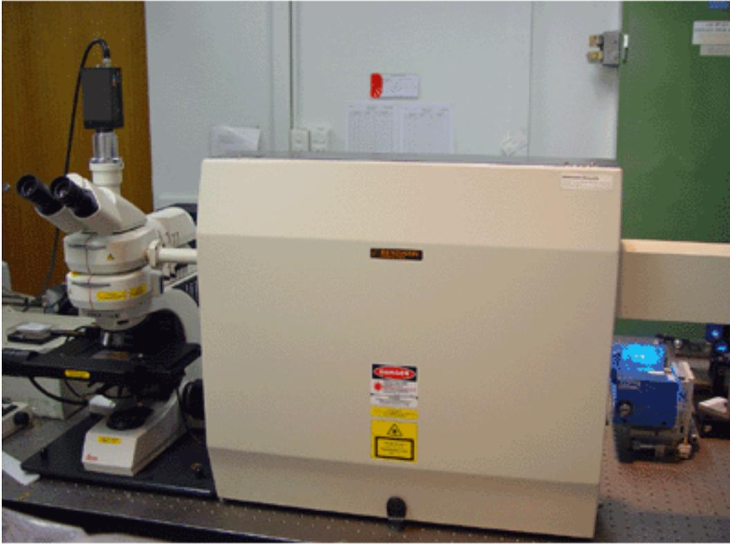
**Figure 11: Renishaw 2000 Raman Spectrometer**
