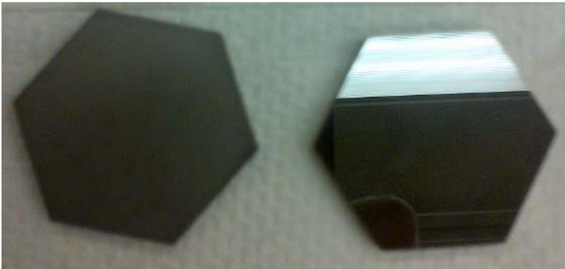
**Figure 4: As-fired (left) and Polished SiC Specimens**
