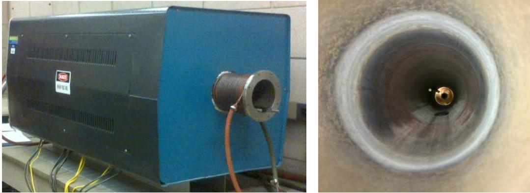
**Figure 7: High Temperature Furnace Equipped with Vacuum Pump**
