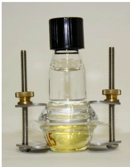
Figure 11. Experimental set up of in vitro release in glass cell with dialysis membrane.
