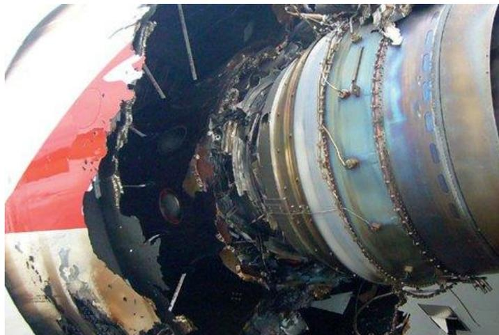
Figure 2: Disk burst on a Qantas A380
