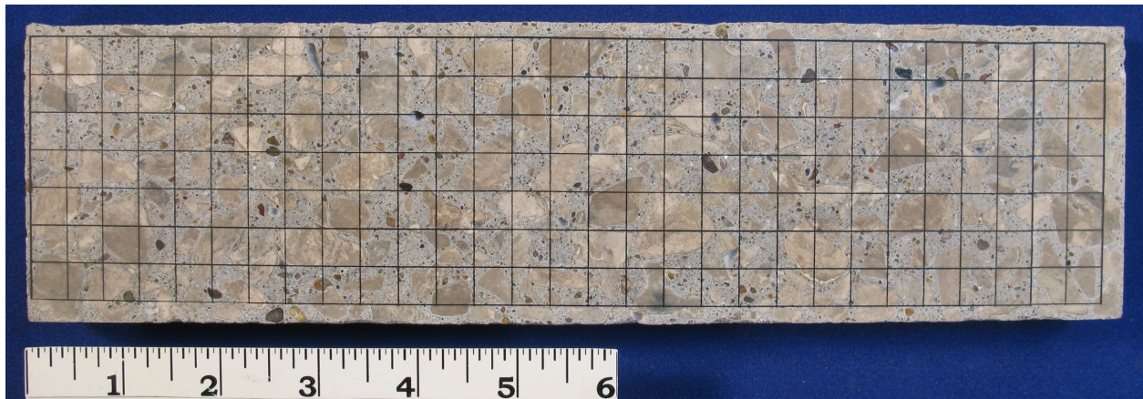
Figure 7 Specimen with DRI grid paper adhered to lapped surface
