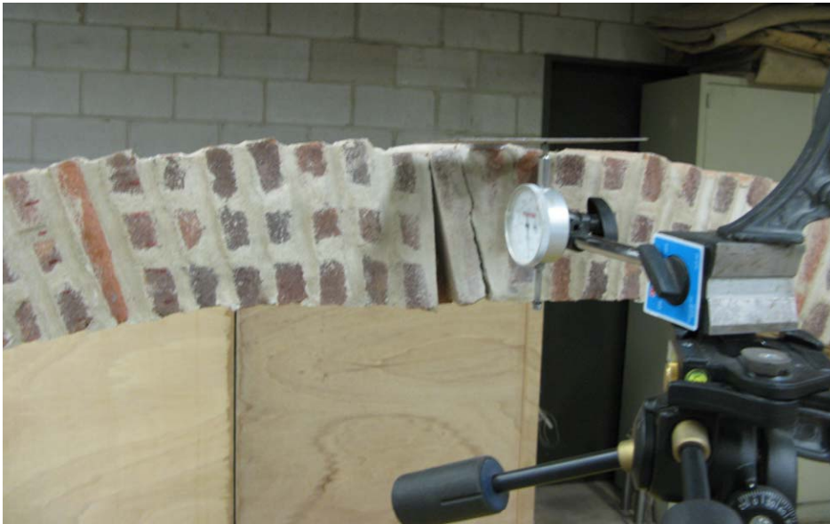
Figure 69. Hinge formation at crown.
