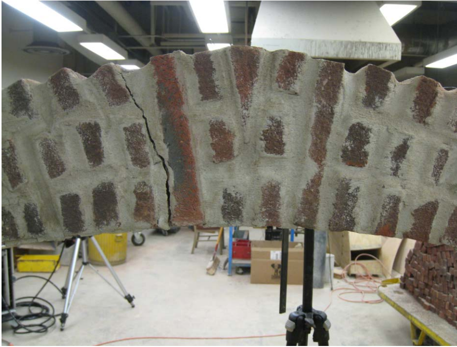
Figure 56. Fully cracked hinge at crown (located 2 courses from center).
