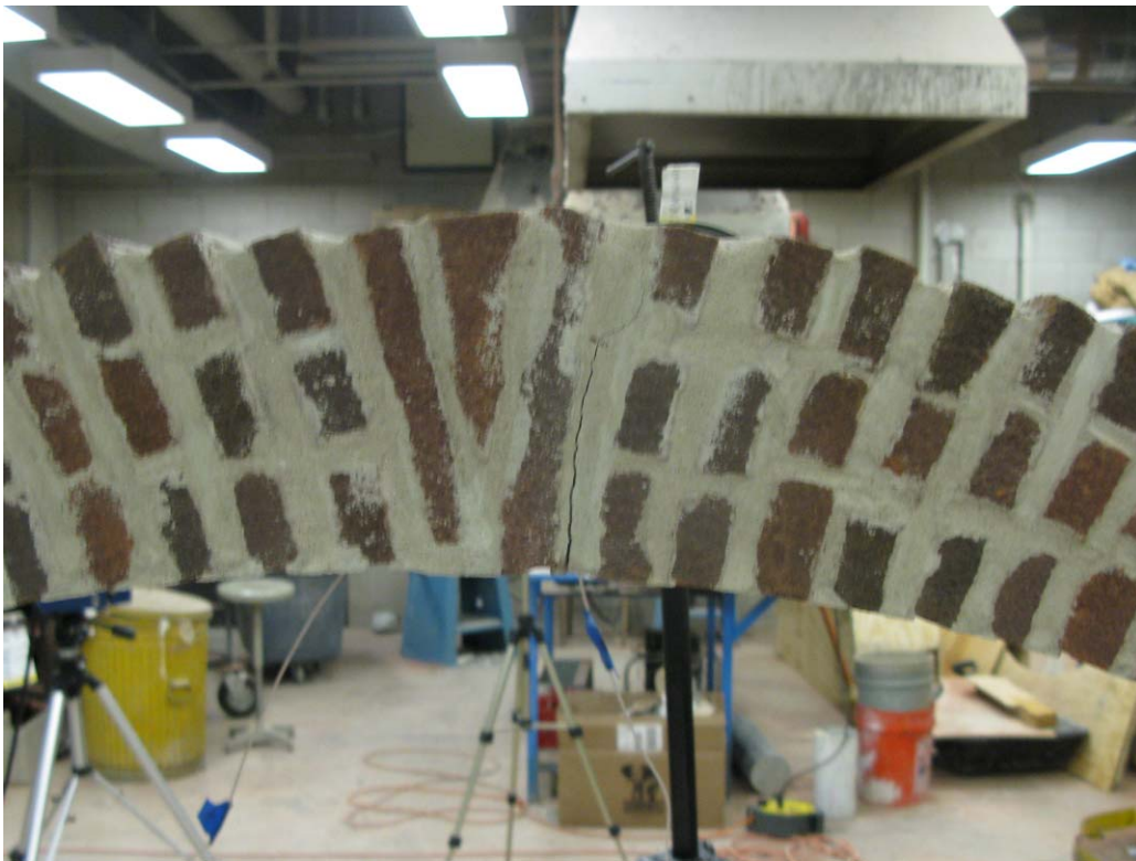
Figure 50. Hinge formation just off center of crown.
