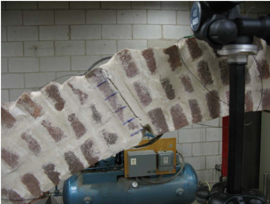
Figure 63. Crack condition after repetitive test cycles.
