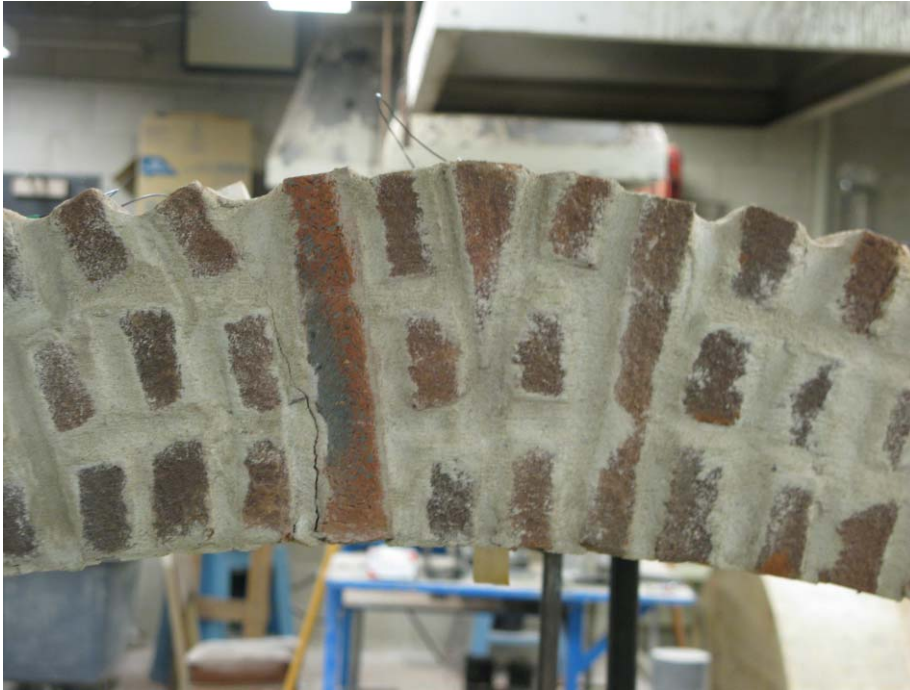
Figure 55. Initial hinge formation at crown.
