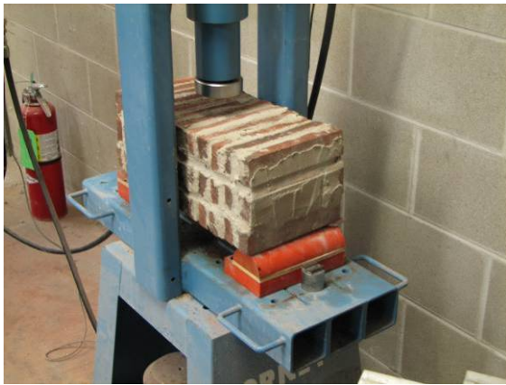
Figure 46. Modulus of rupture test setup.
