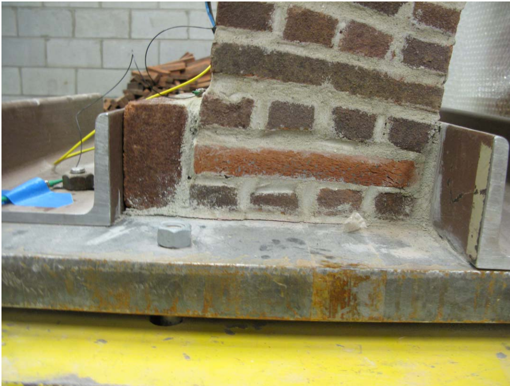
Figure 51. Typical hinge formation at support.
