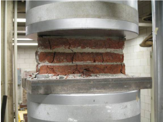
Figure 44. Masonry compression tests.
