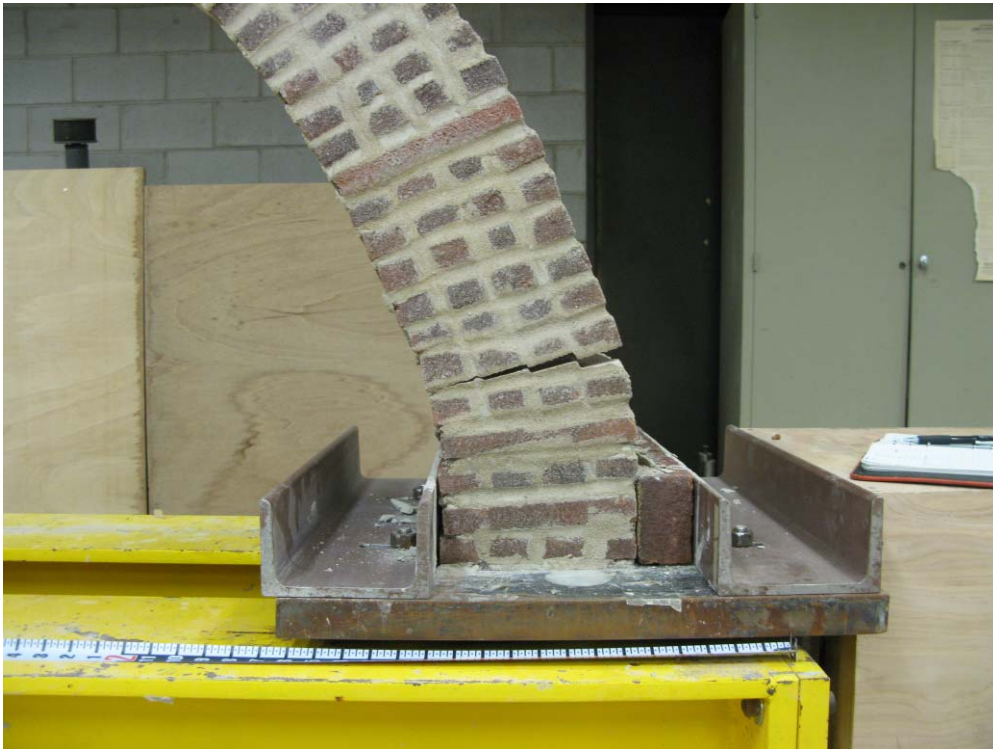
Figure 67. Hinge formation at right support.
