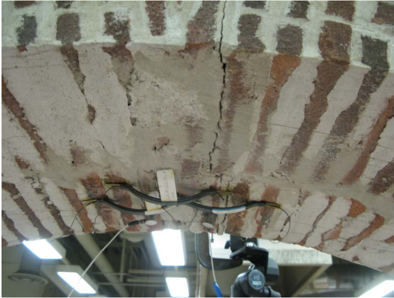
Figure 49. Crack at crown being measured by fiber optic crack sensors.
