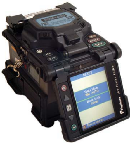
Figure 23. Core alignment fusion splicer.
