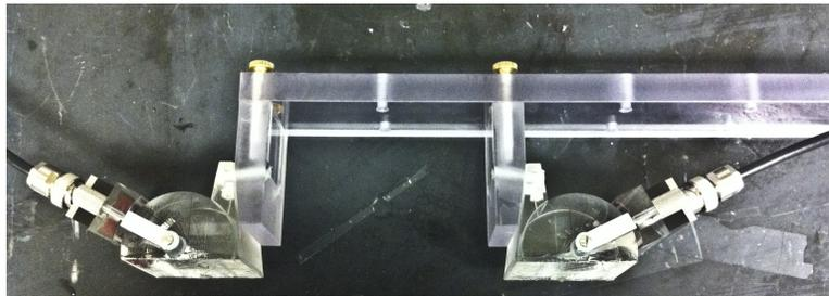
Figure 12. Constructed Wedge Separation Handle
