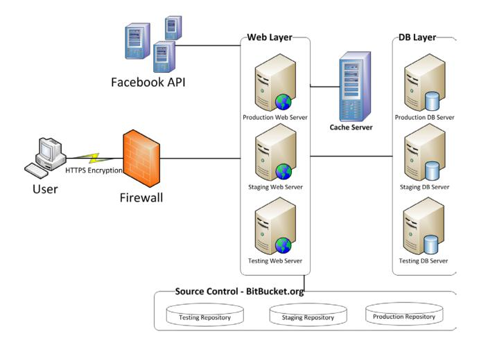
Figure 8: Architecture used for development and development of the prototype.
