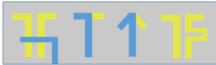
Figure 16 Different planar dipole structure as feed for DRA
