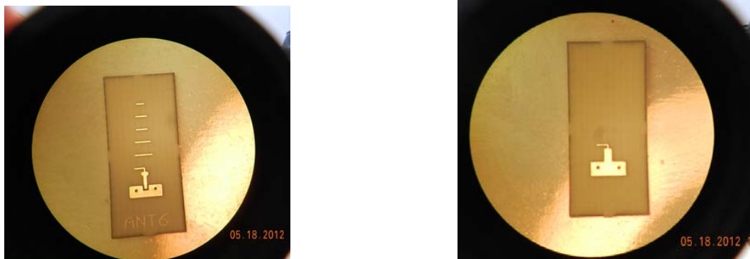
Figure 47 Top and bottom layers of fabricated antenna
