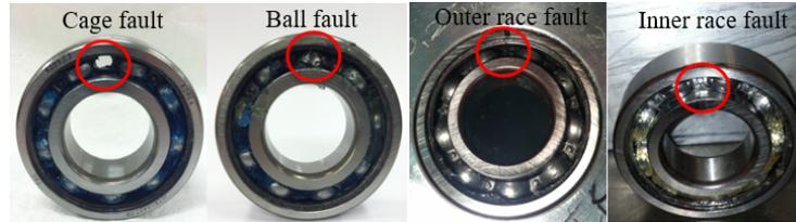
Figure 5.2. The steel bearing with seeded faults
