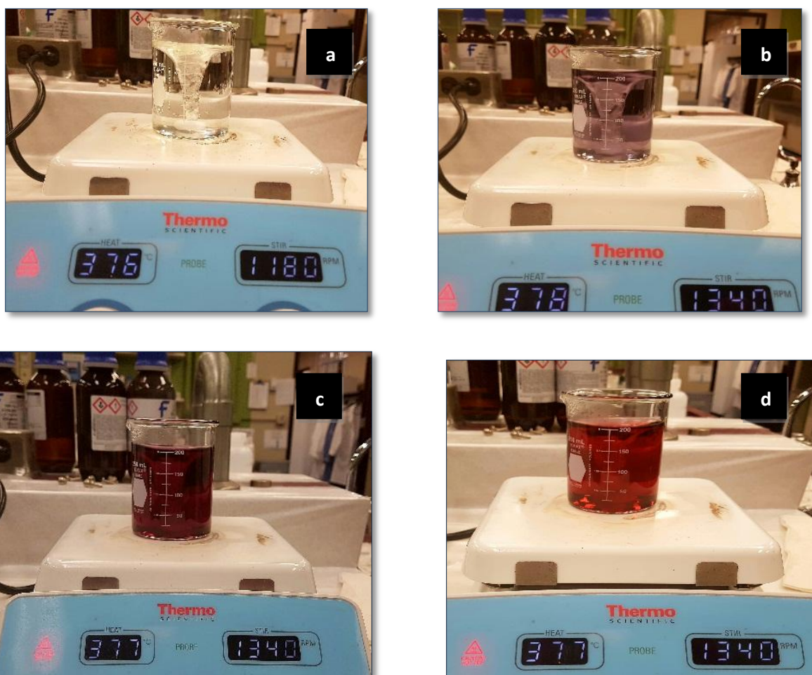
Figure13 - Preparation of Colloidal Au NPs by sodium citrate method
