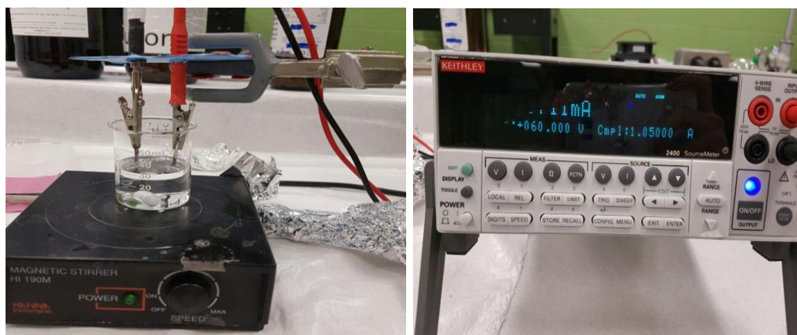
Figure12 - Working station for TiO 2 NTs Anodization
