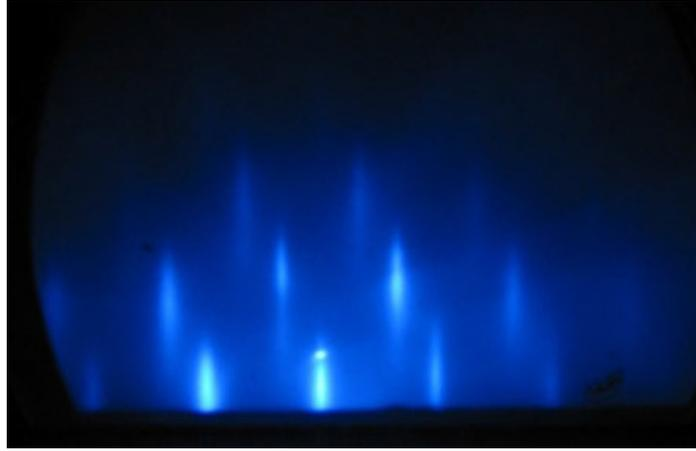
Figure 29: RHEED pattern of GaAs substrate following oxide desorption.
