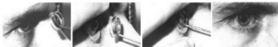
Figure 3: Scleral contact lens for eye-tracking, reprinted with permission [15].
