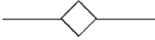
Figure 12: Springpot model (single fractional element).
