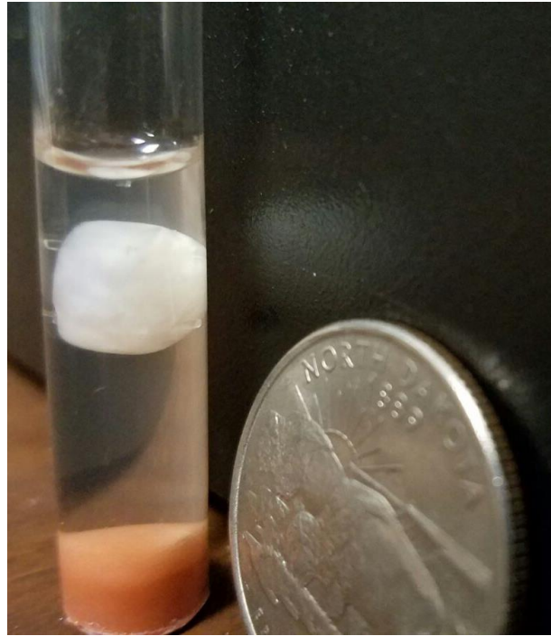
Figure 16: Picture of the anisotropic phantom inside the test tube. Externally the transparent gelatin matrix, inside the PVA matrix with four Spandex fibers inside positioned horizontally.
