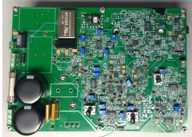
Fig. 30. Fabricated prototype of the proposed closed-loop active gate driver along with the clamped-inductive test circuit of Fig.26. A part of the board is used to derive the results. Rest of the board is used to derive the results of chapter four, ©2015 IEEE.
