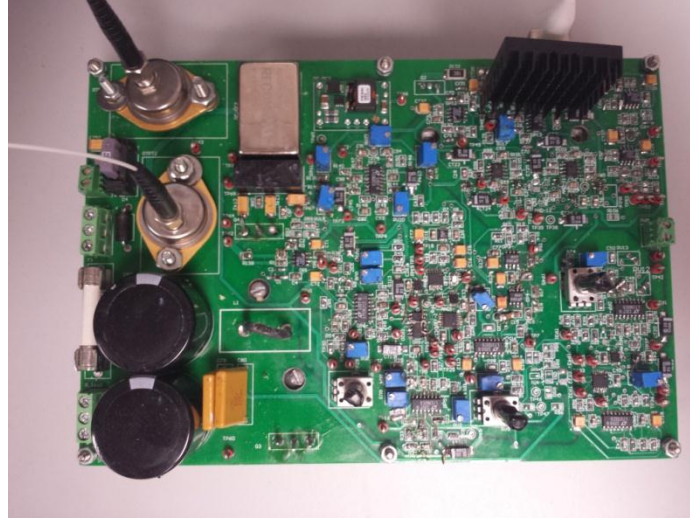
Fig. 45. Fabricated prototype of the proposed control scheme with the clamped-inductive test circuit of Fig. 35.
