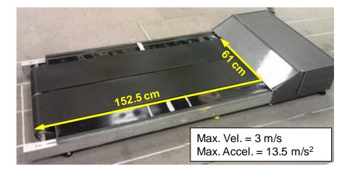
**Figure 6**. The microprosser-controlled, stepper motor-driven, dual-belt treadmill (ActiveStep<sup>TM</sup>, Simbex, Lebanon, NH).
