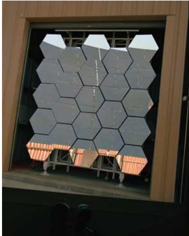
Figure 5: Example of hexagonal-shaped mirrors heliostat [28]
