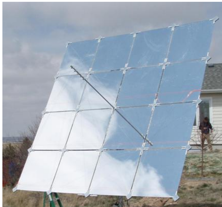
Figure 2: Example of canted-glass mirror heliostat [25]
