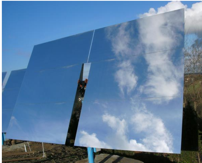
Figure 4: Example of flat, multiple mirror heliostat [27]
