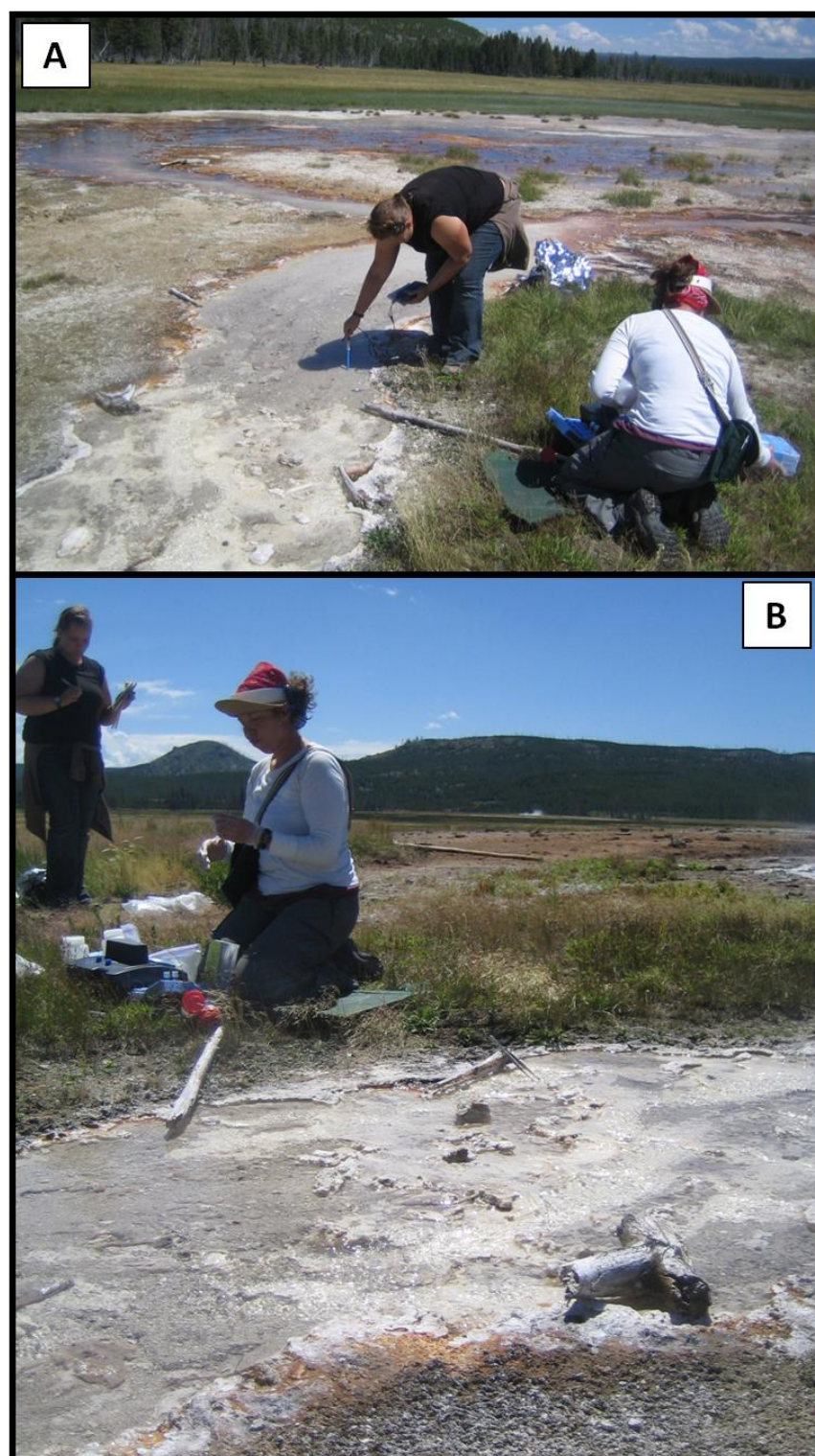
Figure 13. Geochemical sampling at “Bison Pool.” A. Collecting pH and temperature measurements; B: Analyzing fluid chemistry using portable field spectrophotometers and reagents.
