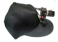
Figure 5: A wearing prototype for acquiring different sources of data
