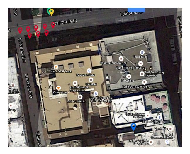
Figure 48: Sample localization result for query image in set 1 in Fig. 47: Noisy query position from GPS (blue), Position of the best matches (red), actual (green) and estimated positions by proposed method (yellow)
