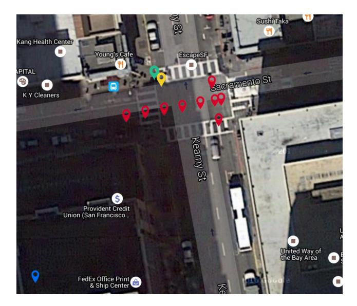
Figure 50: Sample localization result for query image in set 2 in Fig. 49: Noisy query position from GPS (blue), Position of the best matches (red), actual (green) and estimated positions by proposed method (yellow)
