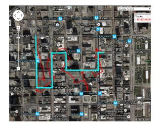
Figure 1: Sample trajectory saved by a smart phone (pure GPS) shown by red and ground truth by Blue
