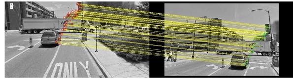
Figure 21: Inliers found after applying Homography verification
