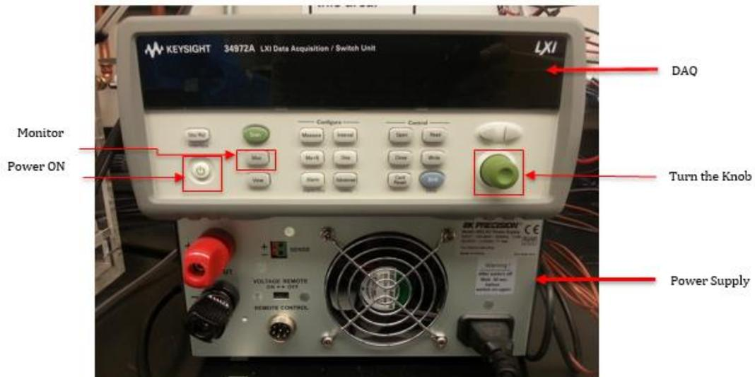
**Figure 22. Data Acquisition System.**
