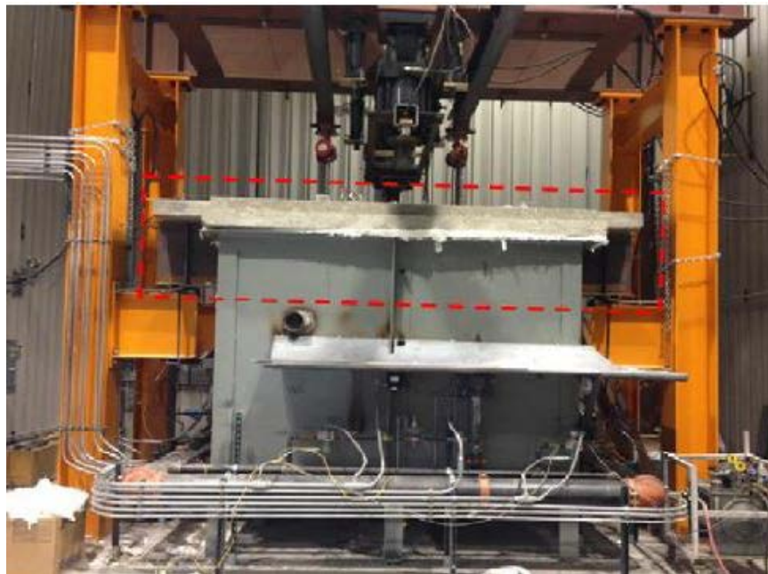
Figure 3-6. Steel girder placement in the furnace. Adopted from (Aziz et al., 2015)
