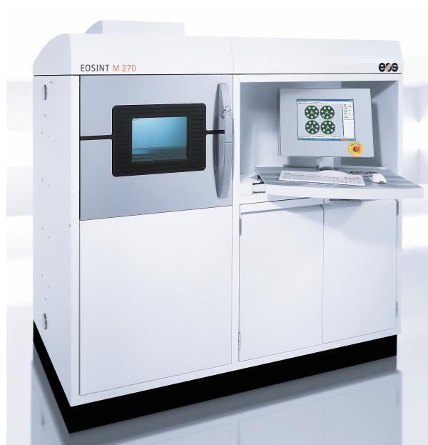
Figure 14: EOSINT M 270 system for Direct Metal Laser Sintering (DMLS), source: EOS.
