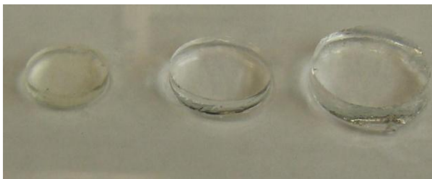
Figure 2.3 Hydrogels at equilibrium swelling. From left to right: PEGDA 3,400, PEGDA 10,000 and PEGDA 20,000. All hydrogels are at 15% w/v initial macromer composition and were originally 8 mm in diameter.
