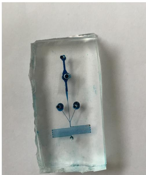
Figure 2.7. Image of the islet perfusion chamber mixer device.
